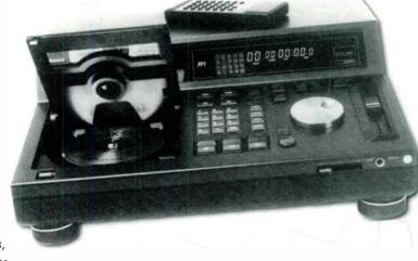
With its heavyweight cast zinc chassis and separate transformers for analogue and digital sections, Technics' SLP1200 CD player makes a fine second-hand buy.
