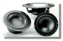
non-reflecting dustcaps minimise distortion created from edge interference. **Peerless** began by reinventing woofer cone material from the ground up, by laminating multiple material layers of differing physical charateristics, **Peerless** engineers created a combination that reinforces the best qualities of each material. Thus the 'Composite Sandwich Cone was born.
