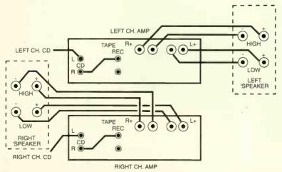
How to wire up two integrated amplifiers for bi-amping. Because both amps are working with mono signals, the right channel CD player output can be plugged into the amp's left 'CD input' socket as shown.
