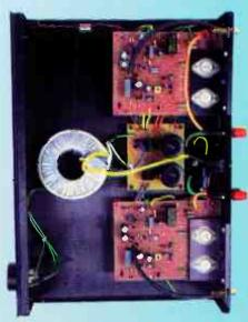
The Tornado I power amp is tidily laid out inside, its power supply capacitors and rather small mains transformer clearly visible.
