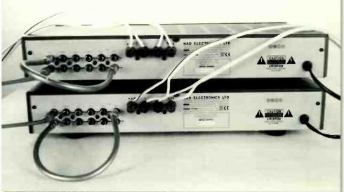
One way to bi-amp using two amps which lack separate 'pre-amp out' and 'power amp in' sockets.
