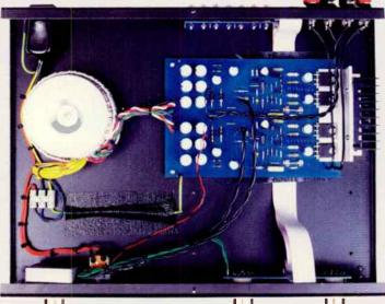
Simplicity is the name of the game with the Mistral Integrated, almost all the components being mounted on a single, small circuit board.
