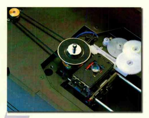
sing Parasound's C/BD-2000 is a bit like using a record deck. Slipping back the smoked Perspex transport cover, you have to put the disc over the spindle and then place the surprisingly heavy puck on top. By the way, don't forget about the puck. The transport works whether it's used or not, and leaving it off can result in the disc spinning crazily inside the machine.
