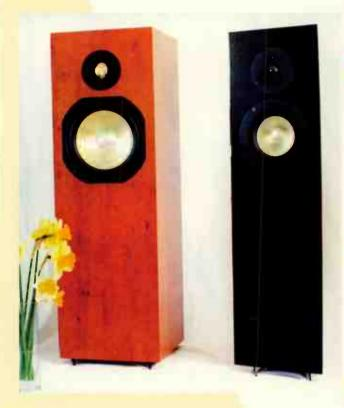
Making up the driver complement for the 300 is Audax's high quality piezo gold dome tweeter and a 180mm mid/bass driver with an anodised spun aluminium cone. This crosses over through a simple, first-order network at 6kHz. With a braced cabinet hewn from 25mm MDF and veneered inside and out, the Concept 300 will set you back £1800.
