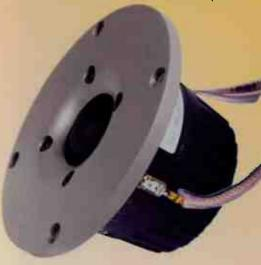
Precious metal - The concert 8's tweeter is wound with pure silver wire and uses a solid zinc cast face plate to reduce resonance.
