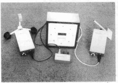
The three sensor heads plugged into the rear of the display unit.
