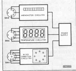
Fig. 4. Overall block diagram for the EE Weather Station displays.
