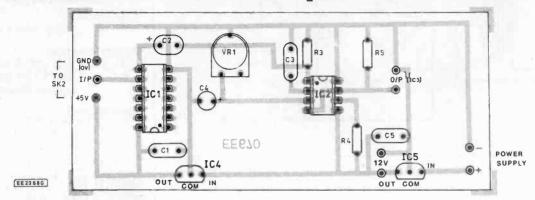
Fig. 9. Printed circuit board component layout and full size copper foil master pattern (below). Connections for the opto-switch X1 and regulators IC4/IC5 are shown below right.
