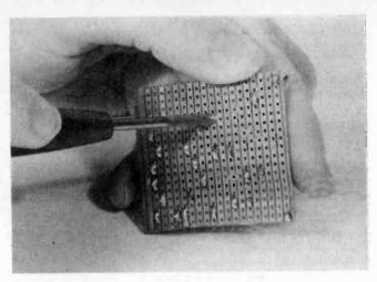
Stripboard (or Veroboard) tracks can be cut using the special tool available or a small (7mm or 8mm) hand held drill hit
