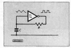
Fig. 3. Simplified Schmitt trigger inverter oscillator circuit.
