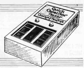
A low-cost, handheld audio/visual unit which can identify short, open and working capacitors quickly and with a minimum of fuss. Also gives some indication of leakage current, especially useful for electrolytics and for diode and transistor junctions.
