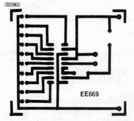
Fig. 10b. Printed circuit board component layout for bargraph display using the LM3914 i.c. and not the module.
