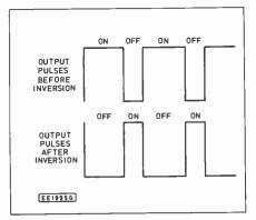
Fig. 2. Output pulses from the timer before and after inversion.
