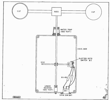
Fig. 11. Mechanical details for the Anemometer head.
