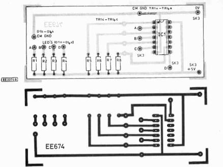
Fig. 13. Printed circuit board component layout and full size master pattern for the wind vane head.
