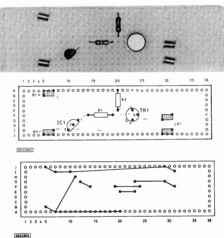
Fig. 2. Easiwire bổard component layout and details of the underside wiring. Note that a lead from the negative of battery B1 should be taken to one side of push switch S1 and a lead from the positive connection of B2 to the other terminal of S1.
