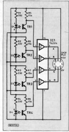
Fig. 12. Complete circuit diagram for the two sections of the Wind Direction Indicator. The connection details for the diodes and phototransistors are shown below.
