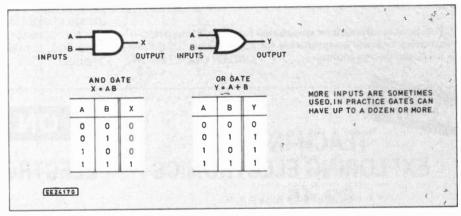
Fig. 3.10. The AND and OR basic functions and gates. Two-input types are shown.
