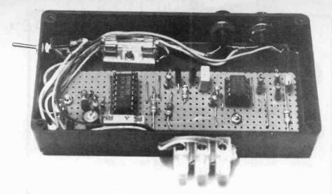
Completed unit showing positioning of components within the plastics case. All wiring should be at least 3A rated auto-type cable.
