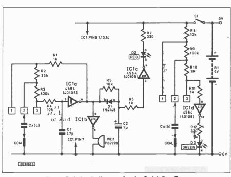
Fig. 4. Full circuit diagram for the Quick Cap Tester.
