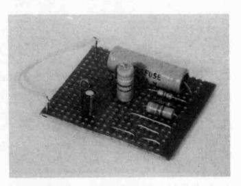
Some cheap components and a piece of stripboard will enable you to practice soldering.
