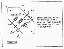
Fig. 3. Top view of the inductor with winding details
