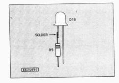
Fig. 5. Connection of R5 and D18.
