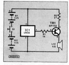
Fig. 1. Complete circuit diagram for the Tune Generator.
