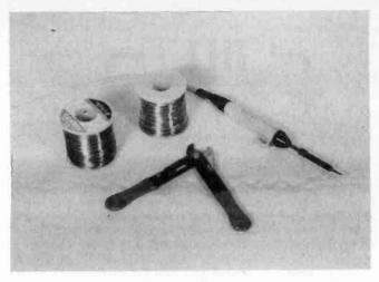
The basic soldering equipment; two sizes of solder, a 17W iron fitted with a miniature bit and combined wire cutters/strippers (these are not ideal for circuit board work).
