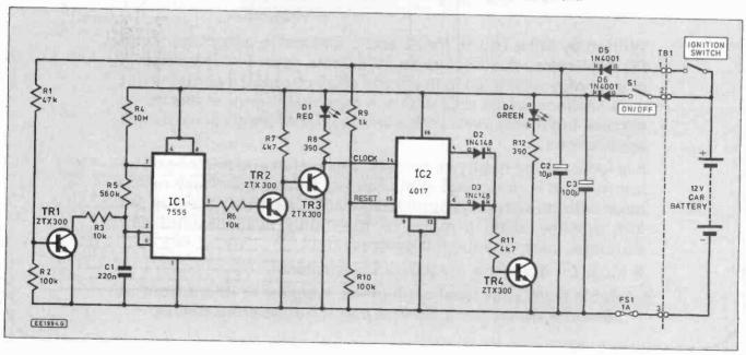
The operating current of D1 is limited to the correct working value by resistor R8.
