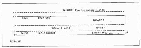
Fig. 3.8. Digital circuit voltages. Most circuits and chips are quite tolerant, fortunately.
