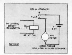
Fig. 3.6. Relay contacts included in the motor circuit
