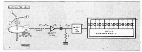
Fig. 1. Block diagram for the Electronic Anemometer (wind speed).
