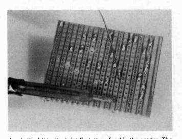
Apply the bit to the joint first, then feed in the solder. The joint should be made in a couple of seconds.
