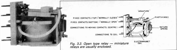
Photo of an open type relay
