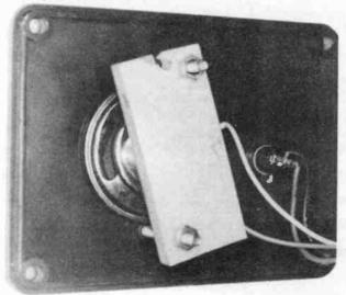
The completed Tune Generator showing the speaker "grille" and push switch S1.
