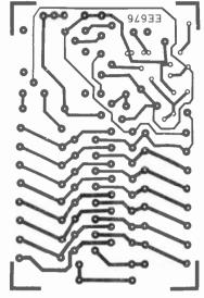
Fig. 4. P.C.B. layout and wiring and the track pattern, shown the correct size above.
