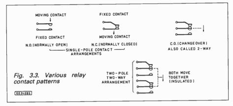
The one in your kit is a miniature type which can be connected to the breadboard with connecting wires, or possibly plugged straight into the breadboard. Switch off, and carefully insert it so that the coil is in the collector circuit INSTEAD of the lamp (Fig. 3.4). Then see if the relay "clicks" as you make the current change by covering (completely) and uncovering the cell as before. Check your circuit carefully if necessary. These relays are designed for a 5
