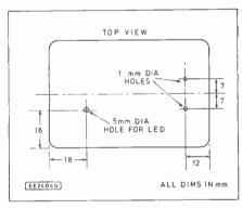
Fig. 6. Case drilling details
