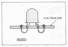
Fig. 6. The leads of diodes D2 and D3 are passed through one set of holes and soldered to adjacent pads, see Fig. 5.
