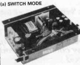
Z660 Astec switched mode PSU Type AA7271.
