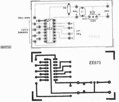
Fig. 14. Component layout and full size master pattern for the wind direction display board.
