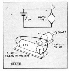
Fig. 3.5. Basic motor/battery circuit
