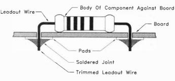
Fig. 1. Mount components with their bodies flat against the board. The solder should flow nicely over the pad and leadout wire as shown. If the component leads are bent slightly (in line with the copper track) they will hold the component in place but should not prevent later removal.
