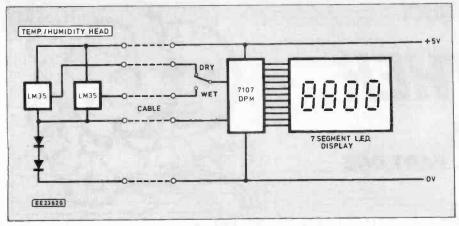
Fig. 3. Block diagram for the Temperature/Humidity unit (Part 2 — next month).
