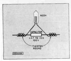
Fig. 7. Simple test circuit
