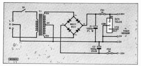
Fig. 6. Circuit diagram for the dual power supply for the EE Weather Station.
