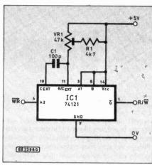
Fig. 3. A monostable circuit which generates a WR signal from the R/W line. An inverter is all that is needed to produce a suitable AD signal.
