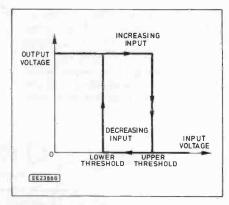
Fig. 2. Graph of the Schmitt trigger threshold levels.
