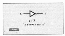
Fig. 3.9. The NOT gate, also called an INVERTER
