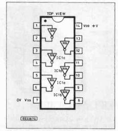
Fig. 1. The 4584 (40106) Hex Schmitt trigger inverter pinout details.
