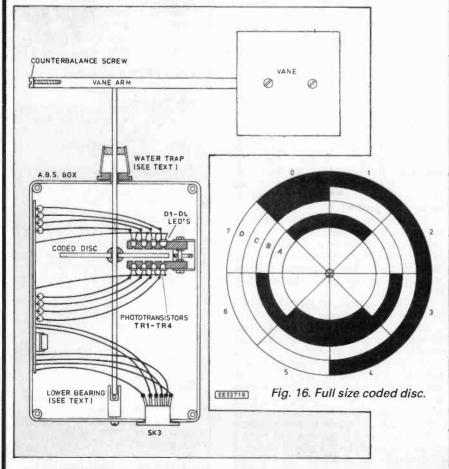
Fig. 15. Mechanical details for the Wind Direction vane head. The sensor bracket holding D1-D4 and TR1-TR4 should be adjustable for aligning with the coded disc.
