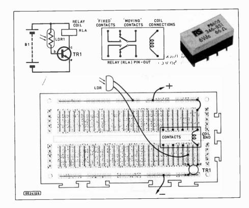
Fig. 3.4. Relay control using an LDR via a transistor
