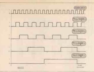
Fig. 3.13. Timing diagram for the circuit of Fig. 3.12.
