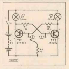
Fig. 7.1. Experimental circuit diagram for a bistable multivibrator.
