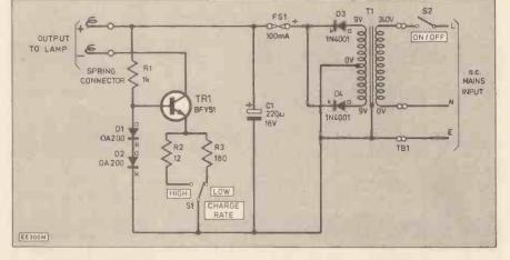
Fig. 1. Complete circuit diagram for the mains-powered version of the Hand Lamp Charger.
