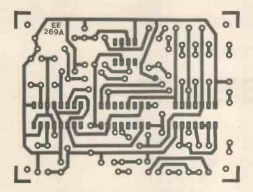
Fig. 3. Printed circuit board layout and wiring.
