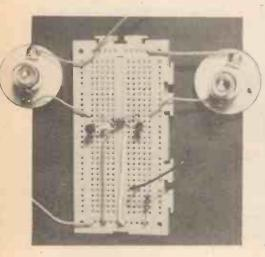
Here we have a circuit that can be in one of two states (point 1 above) and is stable in either state (point 2). This is why it is described as "bi-stable". It can be made to change from one state to another by taking contact A or contact B to a low voltage (points 3 and 4). How it works is explained in Fig. 7.3.
