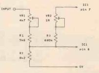
Fig. 3. A zero adjust circuit for a full-scale potential of +5 volts.
