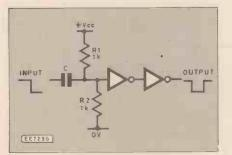
Fig. 3.5. Falling edge triggered negativegoing pulse generator.
