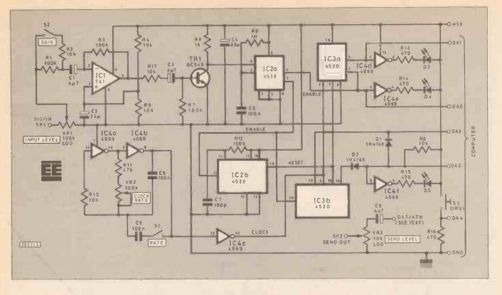
Fig. 2. Complete circuit diagram of the Morse Decoder.
