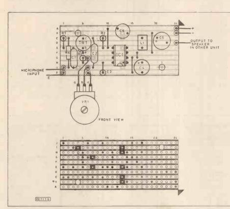
Fig. 3. Component layout, wiring and details of breaks to be made in the underside copper strips of the circuit board. A minimum of two boards are required for this system.
