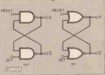
Fig. 3.8. (a) NAND gate RS bistable. (b) NOR gate RS bistable.
