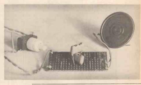
Turn over for details of how to build a Simple Buzzer using an astable multivibrator circuit
