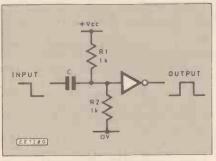
Fig. 3.4. Falling edge triggered positivegoing pulse generator
