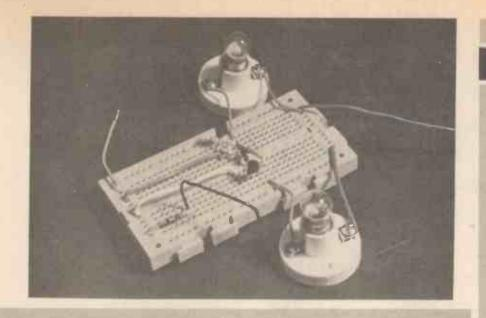
1.8.1 IP2 0 N OFF TR 2 TR1 ON ovo-() STABLE WITH LP1 ON +610 LP1 LP2 TURNED OFF TURNED ON TR2 1 TURNED ON TURNED OFF ovo BASE CURRENT TO TRI SHORT -CIRCUITED TO OV, TURNS TRI OFF CHANGING THE STATE OF OFF TR1 TR2 ON ovo 3 STABLE WITH LP2 ON - SMALL BASE CURRENT - PARTS OF CIRCUIT AT RELATIVELY HIGH VOLTAGE EE7076
