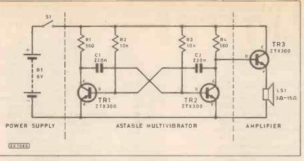
Fig. 7.4. Circuit diagram of an astable multivibrator being used as a Simple Buzzer.
