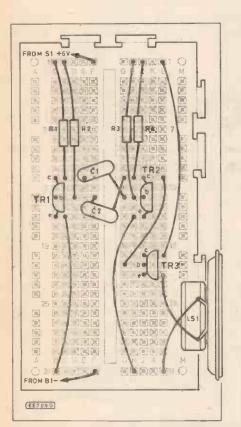
Fig. 7.5. Demonstration breadboard layout for the Simple Buzzer.
