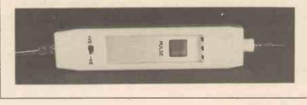
stant,  $R2 \times C2$ , whenever the pulse button, S2, is depressed. With the values specified, the pulse duration is approximately 5ms.
