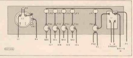
Fig. 3. Wiring of components mounted on the front panel.
