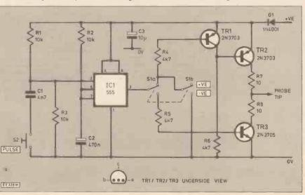
Fig. 1. Complete circuit diagram for the EE Versatile Logic Pulser
