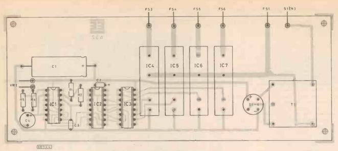
Fig. 2. Printed circuit board layout and wiring.
