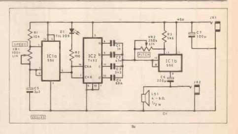
capacitors C1 to C4, with respect of the binary counting. This develops the generation of different notes, the "Pitch" potentiometer VR2 is used to change the frequency of these notes.
