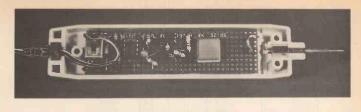
the standard size stripboard used in this series (24 strips of 37 holes); alternatively the remaining unused board from last month's project may be employed.
