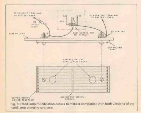
each nut. Check that the head of each fixing makes contact with at least one copper strip and increase the area of contact with a washer if necessary.
