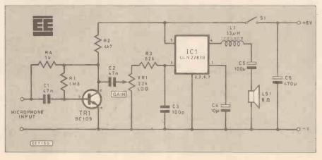
The power supply can be conveniently located anywhere along the route of the connecting cable, where it can be placed out of sight. A 6V lantern battery should be satisfactory for occasional use. In the prototype system the total quiescent current at 6V was about 16mA.
