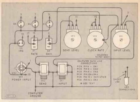
Fig. 4. Wiring of panel mounted components.
