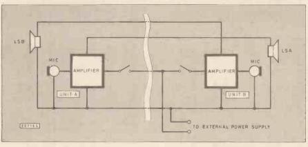
Fig. 1. Block diagram of the operating system for the Hands Off Intercom.
