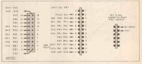
Fig. 5. Connections to the computer.
