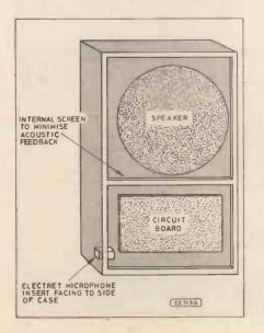
Fig. 4. Suggested arrangement for the wall-mounting unit.
