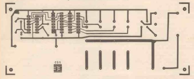
outputs selected to be live by the circuit. It is therefore important to ensure that the cable carrying the "live" power connection to the p.c.b. is capable of withstanding this. load. The outputs from the relays to the fuseholders should be wired in flexible cable capable of carrying a current of 2A. All the remaining connections are required to carry relatively small currents and can therefore be made with relatively small flexible cables.
