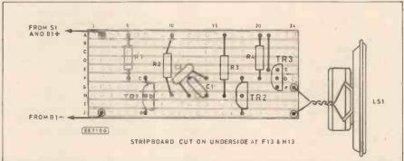
Fig. 7.6. Stripboard component layout for the Simple Buzzer. Remember to make the breaks in the underside copper tracks at points F13 and H13.
