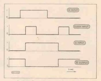
Fig. 3.11. Timing diagram for a D-type bistable.
