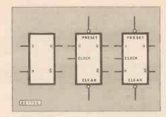
Fig. 3.9. Symbols used for RS, D-type and KJ bistables.
