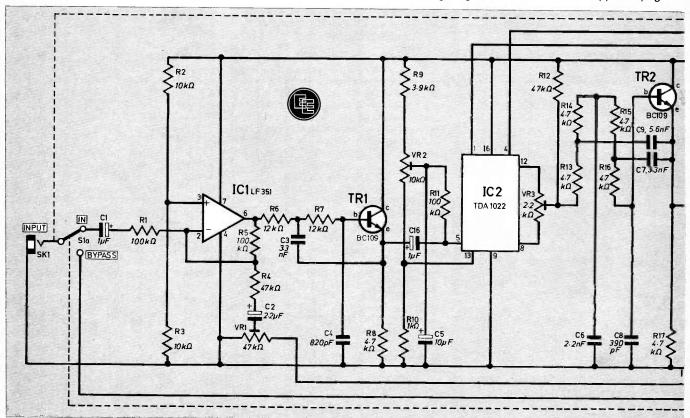
A simple passive mixer, VR3, is used to mix the outputs from stages 512 and 513 of IC2. This is adjusted to balance the outputs and give minimum breakthrough of the clock signal. R12 is the output load resistor for IC2.
