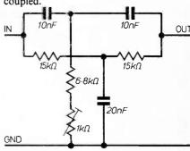
Fig. 6. Circuit diagram for a notch filter used in THD measurements.
