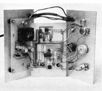
Power supply board mounted on "bushes" on the rear panel.
