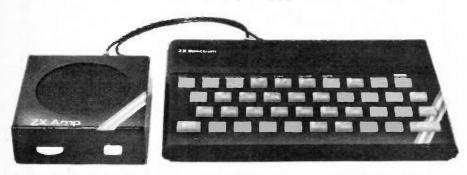
The Beep command is used to produce sound from the Spectrum. Unfortunately the level of this sound is extremely low. In fact, even in a quiet room notes above and below middle-C can be difficult to hear. It was therefore thought necessary that if use of the Beep command was to be fully realised the sound level had to be increased. This was accomplished by the amplifier described here. Apart from being considerably louder the quality of the sound was enriched.
