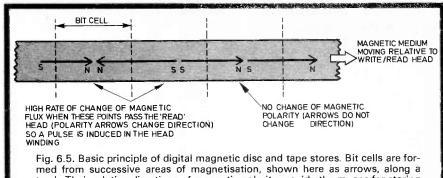
Fig. 6.5. Basic principle of digital magnetic disc and tape stores. Bit cells are formed from successive areas of magnetisation, shown here as arrows, along a track. Their relative directions of magnetic polarity provide the means for storing binary information, at the points where the areas abut (either high rate of magnetic flux change or zero flux change).
