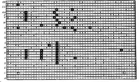
Fig. 4. Component layout, interwiring details and underside of the stripboard showing breaks (41) in the copper strips. The circuit board is mounted on the base of the diecast case and is shown in the photograph on the opposite page.
