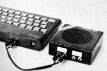
Completed amplifier plugged into the ZX Spectrum.
