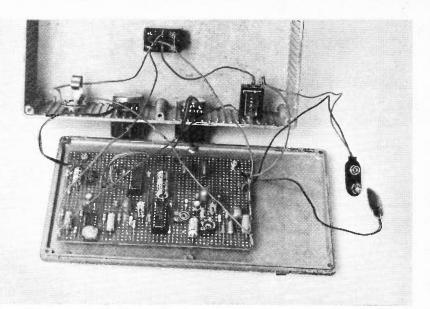
The circuit board mounted in position on the base of the diecast case and side mounted components.
