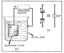
If two electrolytics are connected "back-to-back" (Fig. 1b), one of them is always correctly "polarised", whatever the direction of the applied voltage. Nonpolarised (N.P.) electrolytics are really like this, inside, and are therefore reversible, though hardly true a.c. devices.
