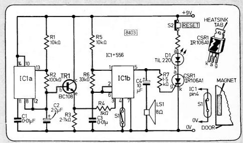
enter or leave the room. Also, as the light emitting diode D1 remains on, once triggered, you have to be able to reset it before entering the room and as you leave.
