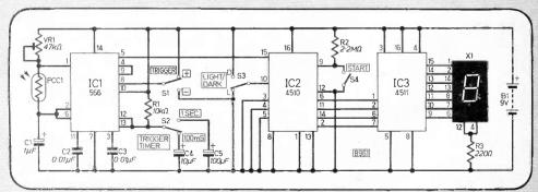
To operate, select how many seconds you want (1 or 0·1), select whether you want it to perform as a light measurer or a darkness measurer, release the start switch until a "0" appears on the display and then turn it back on again, and then pull the trigger switch from negative to positive. You can also adjust the preset
