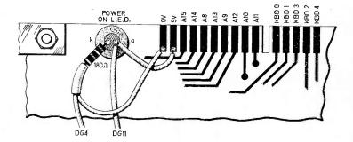
Fig. 4a (upper). Layout of the keyboard switches on the two extreme boards, A and B, and interwiring to each other and the main keyboard p.c.b. with fixing details.
