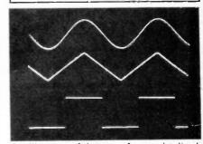
Oscillogram of the waveforms obtained from the Function Generator.
