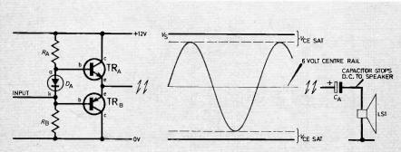
Fig. 1. Diagram showing the output stage of a typical amplifier.
