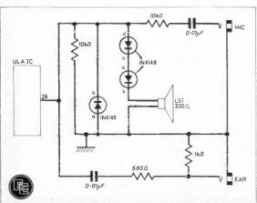
Fig. 2. The complete circuit diagram for the ZX Spectrum Amplifier.
