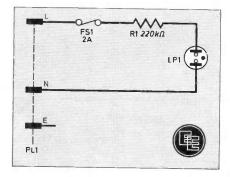
Fig. 1. Complete wiring diagram of Neon Nightlight.
