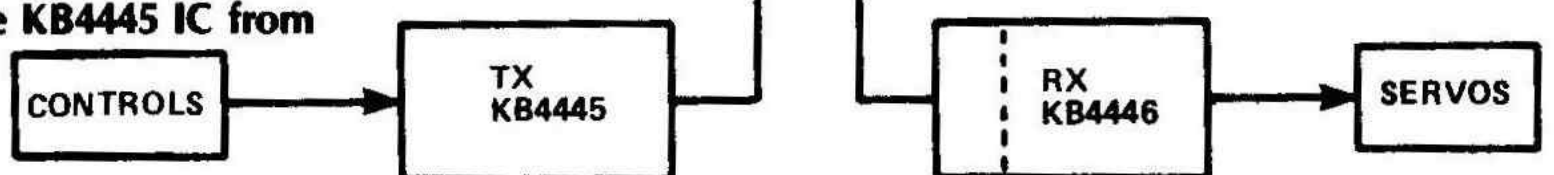
Fig.3 (right) Block diagram of the FM Radio Control link.
