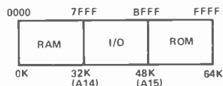
Fig.5 A simple memory map created by allowing the address lines A 14 and A 15 to select the appropriate memory areas. This causes the contents of the selected chip to be 'reflected' through the entire section of memory, but this does not matter provided that you only access the addresses which are connected to a device.
