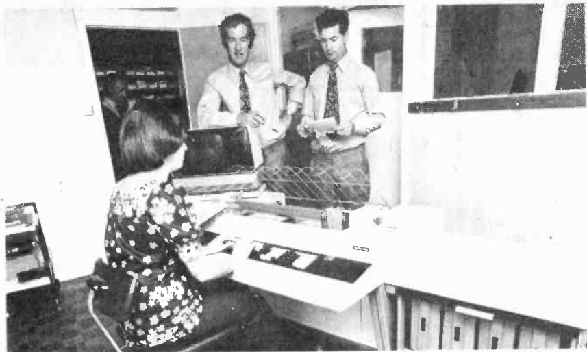
Fig 2. The Willowdale machine in situ. From right to left — floppy discs, keyboard and fast printer and VDU.
