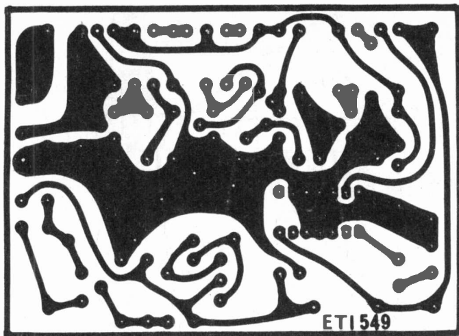
Fig.3 The PCB pattern. Most components other than the meter circuitry is built on this.
