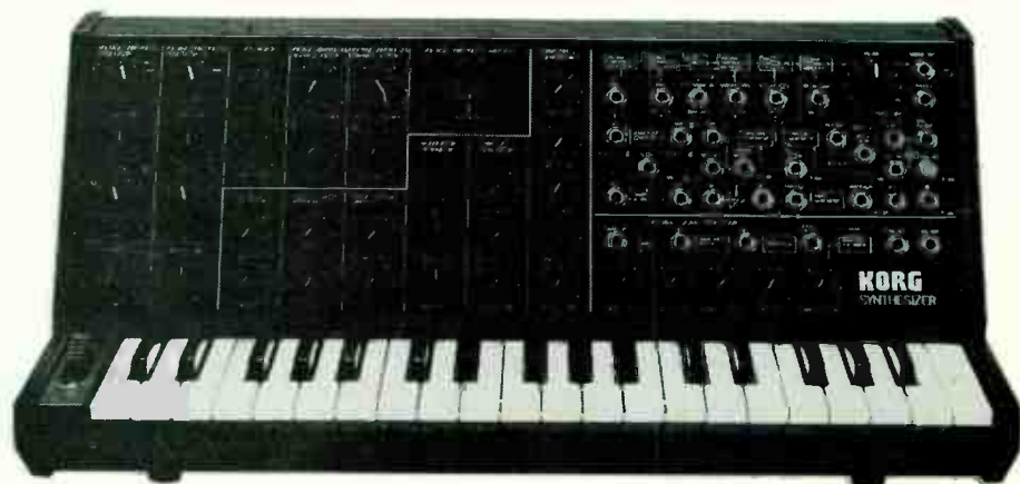
Obsolete but still available in some shops, the Korg MS20 was essentially a modular synthesiser in miniature. Its patching section forms an excellent guide to the principles of analogue synthesis.
