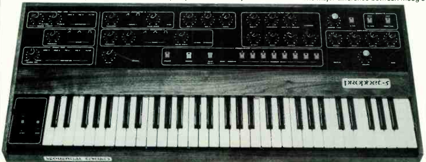
The Prophet 5 – analogue synthesis applied to a polyphonic instrument. Programmable memories made it an overnight success.
