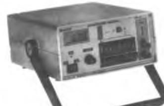
Instrumento preciso e prático, nas escalas de 200 pF, 2nF, 20 nF, 200 nF, 2 μF, 20 μF, 200 μF, 2000 μF, 20 mF.
