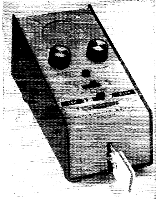
HD-10 shown with new speed-range selector switch mounted just below the original function switch.
