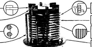
Antenna coil (primary) same low loss construction as secondary.
