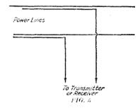
methods of doing this. One of these methods is shown in Fig. 4, where the transmitter or receiver is coupled to the power lines by high-voltage condensers of small capacity, these two being arranged with a protective ground connection. Fig. 5 shows the other method, which merely consists of stringing a pair of wires parallel with the power lines for a distance of a thousand feet or more. These wires act exactly like antennas.
