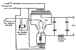
FIG. z = THE CONNECTIONS OF THE POWER SUPPLY UNIT
