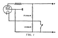
Going a step further, it is possible to subtract the biasing voltage from the plate supply to the oscillator so that when the reduced load on the power supply causes the voltage of it to increase, the amount subtracted will just compensate for this increase and keep the voltage to the oscillator constant even though the load on the power supply may change considerably.
