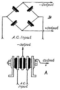
FIG. 5. — THE GENERAL ARRANGEMENT OF A SMALL "ELKON" RECTIFIER USED IN AN "A" SUBSTITUTE IS SHOWN ABOVE
