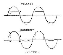
voltage at which the discharge can be maintained is usually about 150 volts below the starting voltage. The voltage across the tube has a peculiar wave-form, shown diagrammatically in Fig. 3. This peculiarity of the tube not only causes a certain distortion of the output wave, but also generates surges, or "transients" in the high voltage circuit which must be absorbed by buffer condensers placed across the transformer secondary. This peculiarity also makes it necessary
