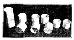
THE STAGES OF MAKING A TUBE BASE. At the left—rod as taken from the mould. Next. slices cut by gang saw. Next, cups as taken from lathe. Next, cup with drilled holes. At the right, finished base with trademark stamped thereon.
