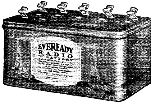
Eveready "B" Battery No. 766. 22½ volts. Six Fahnestock Spring Clip Terminals, giving variable voltage from 16¼ to 22½ volts, in 1¼-volt steps. Length, 6¾ ins.; width, 4¾ ins.; height, 3 3/16 ins. Weight, 5 lbs.
