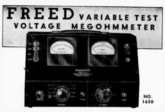
The Freed Type 1620 Megohmeneter is a versotile insulation resistance measurement instrument with a continuously variable DC test potential fram 50 to 1000 valts.
