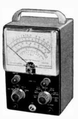
voltage scale provides over 21/4" of scale length per volt measured! Features: modern circuit design for faster, easier construction and stable performance; logical and functional placement of controls for smooth, rapid operation; 1% precision resistors used for high accuracy; high impedance 11 megohm input. Comprehensive construction manual for simplified assembly.
