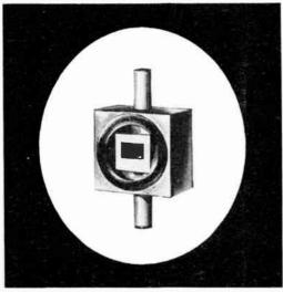
The Philco 1N2792 is a symmetrical, point-contact germanium millimeter - wave diode. It has been designed especially for optimum low-noise mixer operation at 70,000 mc. It is also well suited for long-range space communications and EHF video detector applications over the 50 to 75 kmc portion of the RF spectrum.
