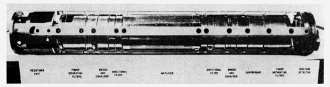
Repeaters such as this are sealed into submarine cables. Amplifying both directions and including directional filters, they will permit bothway transmission through one cable. Some 300 component parts, gold-plated, form its content with a tested life span up to 20 years on the ocean bottom.
