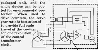
Typical servo repeater/counter device Output shaft that converts synchro data to digital readout.
