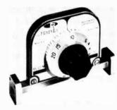
A unique, though simple, new design principle utilizing a variable inserted Narda-Iron cam provides minimum frequency sensitivity and low VSWR over the entire frequency and attenuation range. The direct reading dial is accurately calibrated to within 1 db up to 10 db and 1.5 db up to 20 db over the entire waveguide frequency range. Maximum attenuation exceeds 25 db and minimum insertion loss is under 0.5 db.
