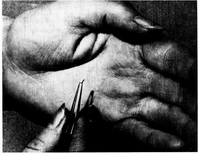
General Electric's newly developed gallium arsenide tunnel diode works at frequencies above 4000-megacycles (4 billion cycles). G.E. expects to make samples available in about 6 months.
