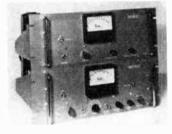
Voiceplex incorporates a novel time division multiplex technique for transmitting and sequentially sampling the two separate channels at a very slow rate. Thus, it may be used without obsolescence of existing equipment or increasing spectrum requirements. Special circuitry is included for generating a new type of high stability synchronizing wave and a sampling system for decoding and separating the two channels. Kahn Research Laboratories, Inc., 22 Pine Street, Freeport L.I., N.Y., U.S.A.
