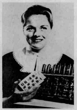
Miniaturization in solid-state data processing equipment can be seen by comparing the printed wiring card (left) used in the new IBM 609 Calculator with a pluggable tube unit (right) used in vacuum tube machines.
