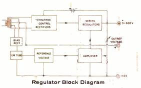
Ripple: less than 1 mv (120c) Regulation: 0.75v for ±10% line change: 0.1v from no load to full load Output Impedance: Approximately  $0.3\Omega$  plus  $10~\mu h$
