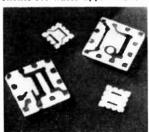
No potting or other mechanical protection is needed, as the ex-tremely hard surface remains impervious to environmental condi-
