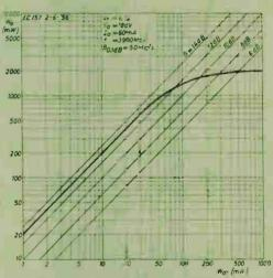
Output power ( $W_a$ ) of the EC157 as a function of the driving power ( $W_{dr}$ ) with lines of constant power gain (G); (I=3900 Me/s.  $B_{0.1\ dB}=50\ \text{Me/s}$ ,  $V_a=180\ \text{V}$ ,  $I_a=60\ \text{mA}$ ).
