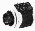
A noteworthy feature of these "high voltage" transformers is a tap which permits operation at 120 volts input with 280 volts output for the VT8H and 240 volts output for the VT8HN (some derating is required for output beyond 120 volts). These high voltage transformers can also be obtained in ganged assemblies to achieve 240-volt, 3-phase operation or 480-volt single phase or 3-phase operation. Request Bulletin 151 from Ohmite Manufacturing Company, 3696 Howard St., Skokie, Illinois, U.S.A.
