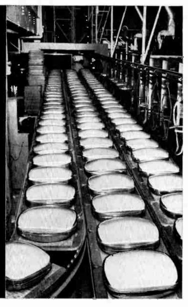
Television set manufacturers are constantly striving to obtain even better video performance from their sets. One way this can now be done is to install new, improved GE picture tubes. At C.G.E., engineers have developed a new screen manufacturing process that produces 20% greater brightness and increased contrast on every GE picture tube.
