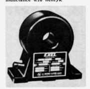
Essentially, an Exel consists of a gapped, strip-wound silicon steel toroid core, wire-wound and imbedded in epoxy compound. The entire assembly is enclosed in a compact phenolic case having two Superior 5-way binding posts for connections. Dimensions are 6" L x 256" W x 534" H.
