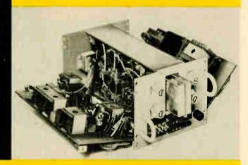
Cover removed to show Channel and Signalling Units — 2 Channels per panel.
