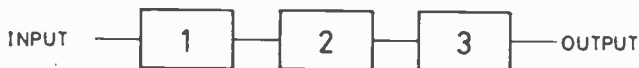
Fig. 3. A chain of bistable counters, with the Q2 collector of bistable 1 connected to the input of bistable 2 and the Q2 collector of bistable 2 connected to the input of bistable 3.
