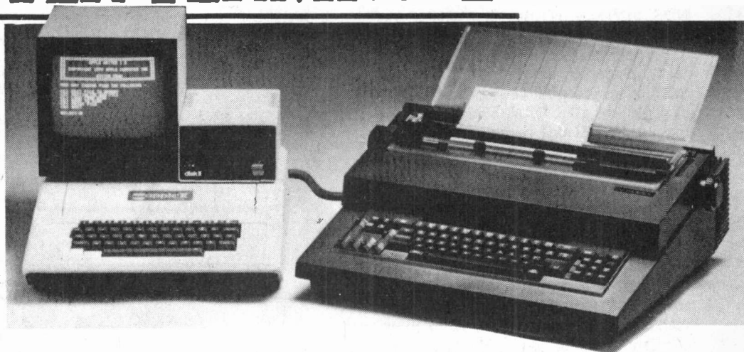
Fig. 1. The NDS 1221 terminal (right) hooked up for use with an Apple II. Even though it's essentially a converted office typewriter, it is nevertheless an effective computer terminal.
