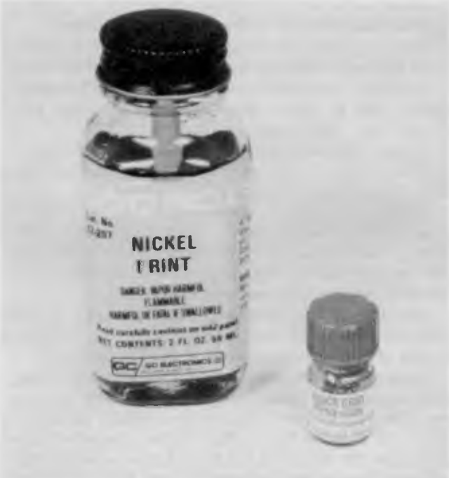
FIG. 4—THESE TWO CONDUCTIVE INKS are low priced, readily available, and suitable for hand application.
