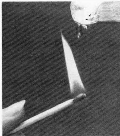
FIG. 9—THE HEAT FROM A MATCH is enough to melt a bar of indium fusible-alloy solder.
