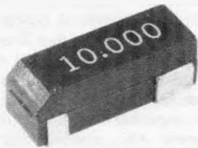
FIG. 14—COMPONENTS SUCH AS CRYSTAL FILTERS, relays, switches, and crystals are available as SMC's. An SMC crystal is shown here.
