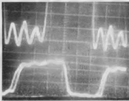
FIG. 3—RINGING ON THE WAVEFORM was finally found to be the cause of the problem.
