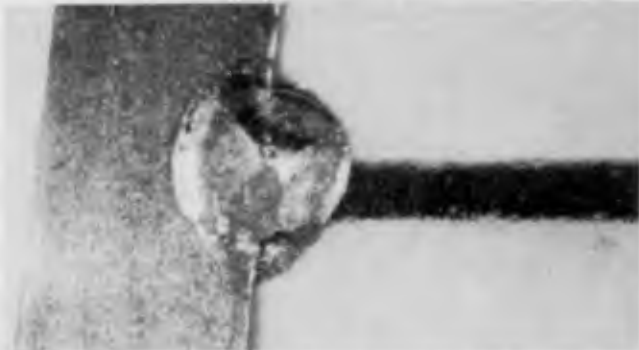
FIG. 4—A DROPLET OF CONDUCTIVE INK connects a graphite resistor to the copper strip.
