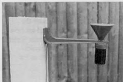
FIG. 6—THE SENSOR ASSEMBLY should be mounted on a long bracket that is screwed to a post. The post should be mounted away from overhanging eaves; and don't mount it under a tree.
