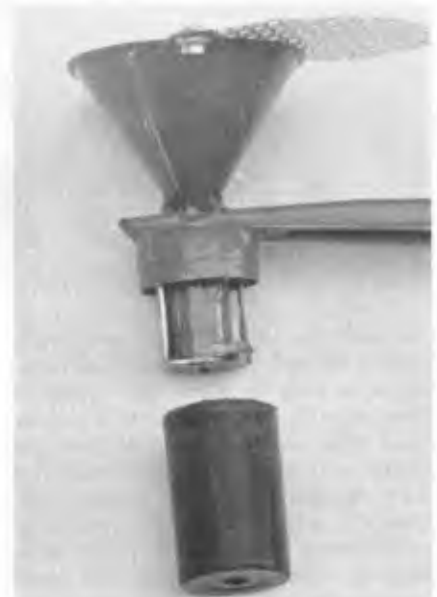
FIG. 4—A 35MM FILM CANISTER provides a water-tight enclosure for the solenoid valve.
