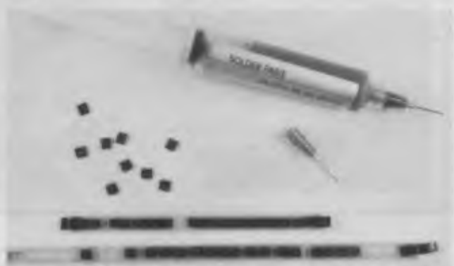
FIG. 3—SOLDER PASTE OR CREAM is available in a syringe. That makes dispensing the paste or cream convenient, once you get the hang of how it's done!
