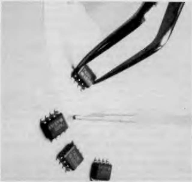
FIG. 3—USING THE TRANSFER METHOD to apply conductive adhesive to the pins of an SO device.
