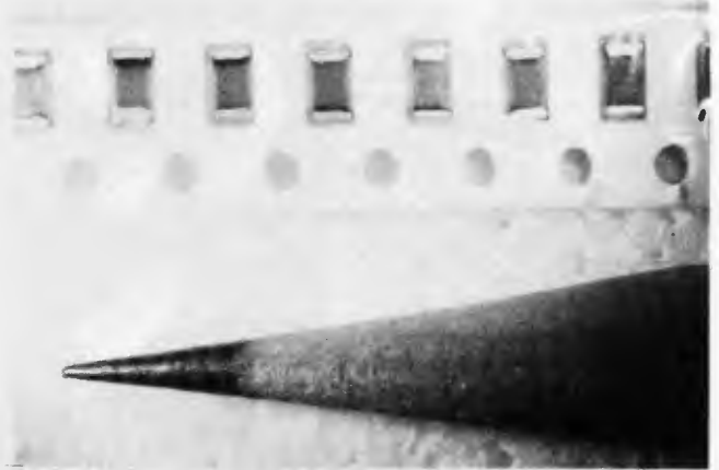
FIG. 4—A STRIP OF CHIP RESISTORS supplied on tape. The pencil point in the photograph is shown for scale.
