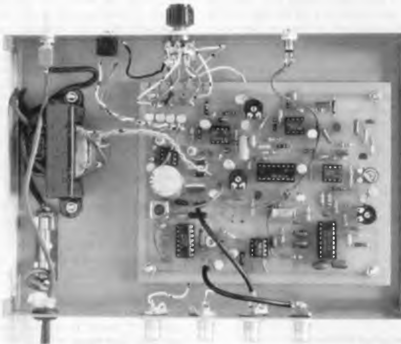
FIG. 7—THE COMPLETED STEREO DECODER BOARD. Next time, we'll show you how to build the circuit shown here.
