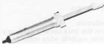
FIG. 7—A SOLDER-SUCKER removes solder from a one-surface component-mounting hole or a plated-through connection.
