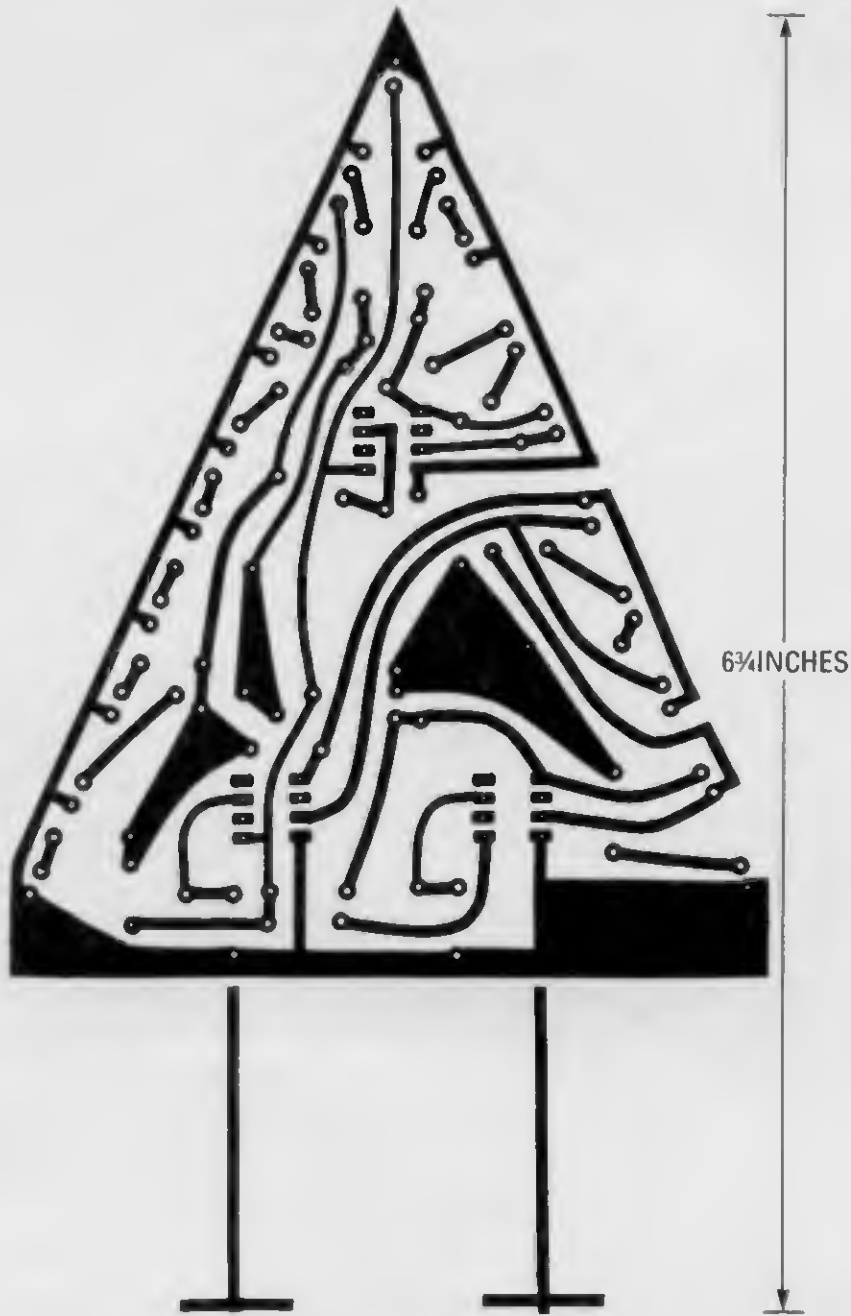
LIGHT UP THE HOLIDAYS with the electronic Xmas tree. The PC board for that project is shown here.
