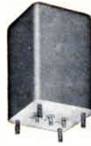
High frequency low pass filter. Zero to 700 KC within 1 db. 1.95 mc to 10 mc 40 db minimum. Source and Load 1000 ohms. Molded flat construction for printed circuit applications. Size: 1 x 2 x 1/2"; Wt: 1 oz. MIL-F-18327B.
