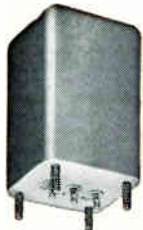
560 \sim Telemetry low pass filter. Available from 400 \sim to 70 KC. \pm 7.5% bandwidth flat to 1 db. Attenuation greater than 35 db beyond the 2nd harmonic of \sim 7.5% frequency. Impedance 47K ohms. MIL-F-18327B. Wt. 0.8 oz.
