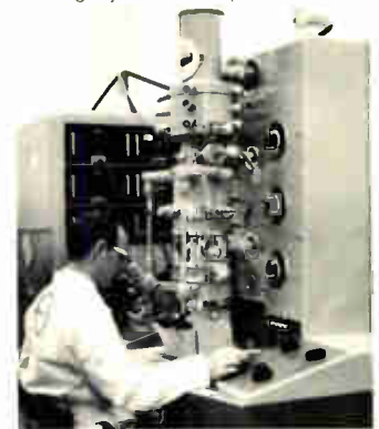
Electron microscope used for epitaxy research
