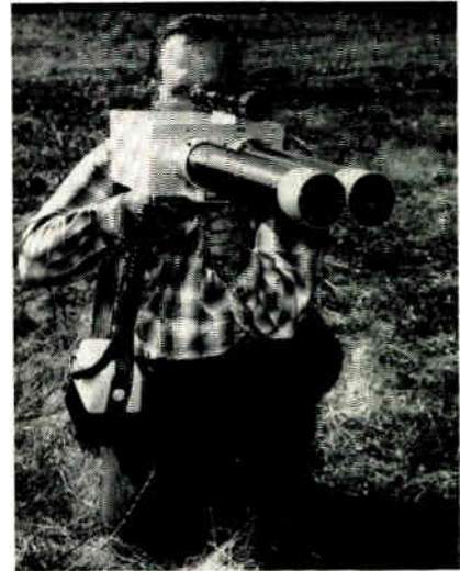
Lightweight and portable, the laser rangefinder makes use of pin-thin beams produced by lasers, and the principles of radar.
