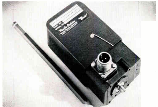
Fig. 4: Gear motor uses a unique rectangular field stack coupled with toroidal field windings. The 1 and 1/4 lb unit delivers 1/10 hp continuous duty 1/4 hp intermittent duty. Unit illustrated incorporates a 3:1 gear reduction and delivers approx. 22 in-oz torque at 3 and 1/2 a, 27 vdc.
