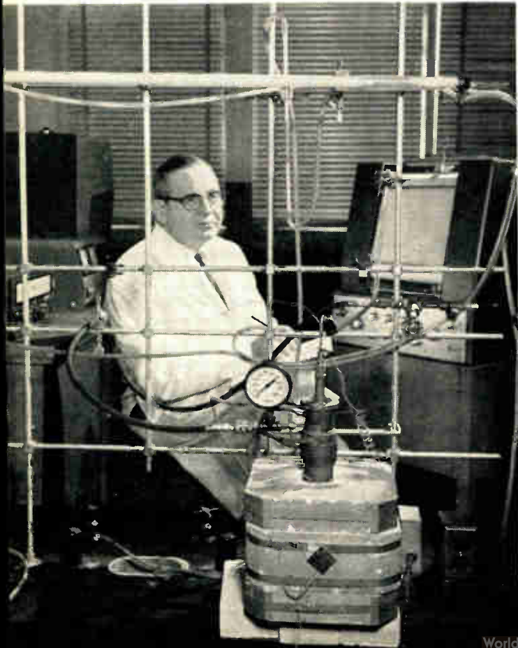
Fig. 1. Dr. B. Agruss, electrochemist at the Allison Div. of General Motors, is shown with regenerative liquid metal fuel cell he invented. Lab model is encased in small furnace in the foreground.
