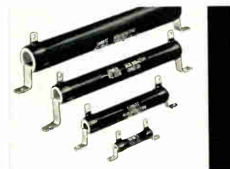
NON-INDUCTIVE: Vitreous Enameled; Wire-Wound; 10, 50, 100, 160 Watts
