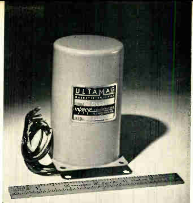
Fig. 9: "One Hundred" line provide up to 43 db polarity reversible gain with zero stability better than 1%. Overload capacity is 1,000% and the units are highly resistant to radiation. Operating Temperatures are from -10 to 180°F. Units measure 4.31 in. High x 2.53 in. dia.
