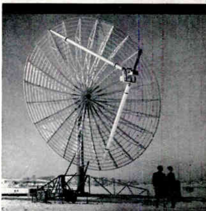
This 30-foot mobile scatter antenna (Model 111) is a completely self contained unit mounted on a steel flat bed trailer. It is easy to assemble, and can be erected by a winch or a hydraulic lifting device. When in transit, all surface panels, hardware, feed supports, guys, etc. nest compactly on the top of the trailer and can be tightly secured in order to withstand transport over rough terrain. The pictures show (1) the antenna completely packed and ready for transit, (2) assembled but not erected, (3) completely erected.
