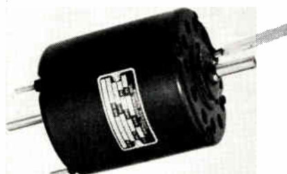
Fig. 7: Universal motor, Model SMZ, develops 1/4 hp, 27.5 v, 11a, 4500 rpm at 30 oz-in. Starting torque is 36 oz-in. It is 4 and 1/8 in. in dia. and about 4 and 3/4 in. long.
