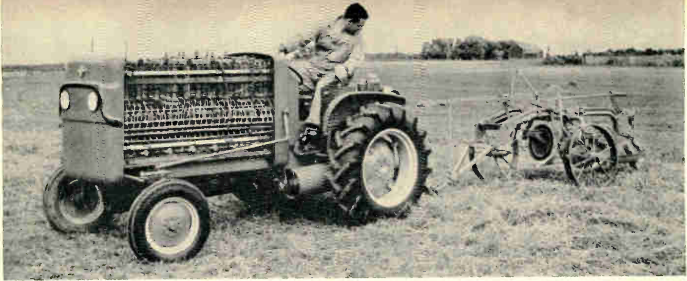
Fig. 10. One thousand and eight Allis-Chalmers fuel cells were used to drive this farm tractor in an experiment conducted in October of 1959.
