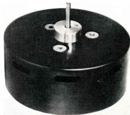
Fig. 2: Precision hysteresis synchronous motor. Motor-induced flutter will not exceed 0.1 rms at 1200 rpm or 0.15 rms at 360 rpm. They will withstand temperature ambients from -32 to 135 C. Applications include tape transports, turntable drives, missile instrumentation, and computer drum drives.
