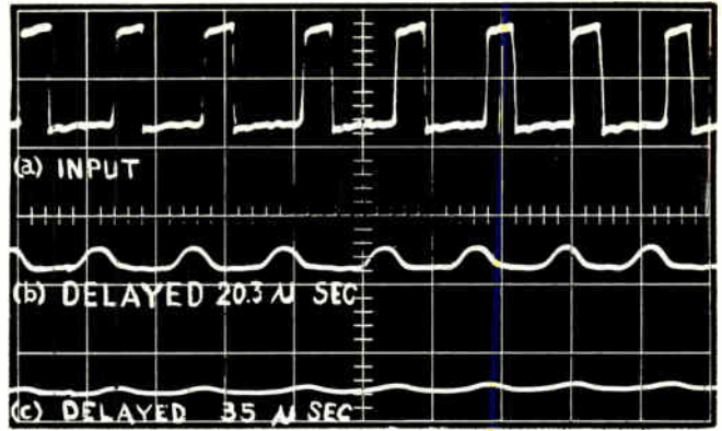
Fig. 3: Pulse deterioration caused by distributed constant line.
