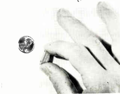
Fig. 3: New design concept of Elgin Indium cell permits variety in shape and size.
