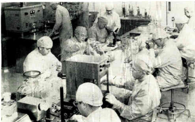
(Left) Assemblers wash, scrub shoes and don nylon uniforms before entering assembly area.
