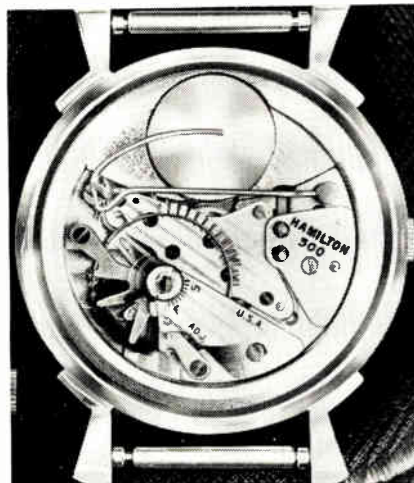
Fig. 7: The new Hamilton electric wrist watch has fewer parts than a wound watch.
