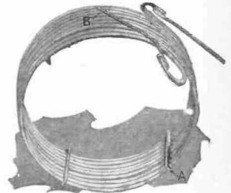
Fig. 5 Above: One of the low-loss coils showing the supporting strips and leads.
