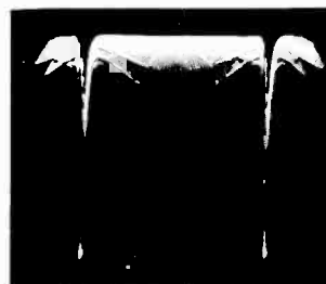
Sync separator output, plate of V4, (pin 3 of 8AW8A) or (L19 of VIFS panel) 36 volts p-p, 60 c.p.s.
