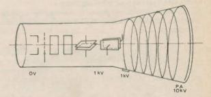
Fig. 4. Spiral p.d.a. (courtesy Enertec Instrumentation Ltd.)
