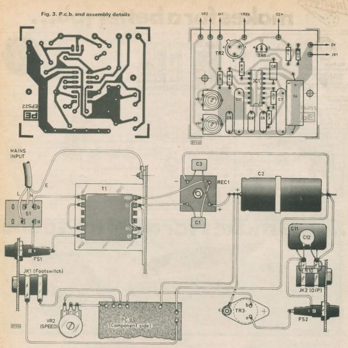
Fig. 4. Interwiring detail
