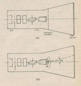
Fig. 5. (a) Mesh p.d.a.; (b) As (a) combined with expansion lens (courtesy Enertec Instrumentation Ltd.)
