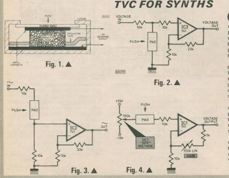
COMMERCIAL performance synthesisers use many forms of man/machine interface. Of these, the pitch-pad is rarely seen on home produced synthesisers. The touch voltage control (TVC) described here enables the pitch pad idea to be applied to almost any synthesiser.
