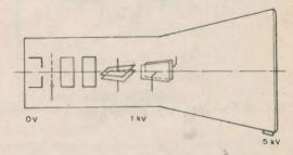
Fig. 3. Single-stage post-deflection acceleration (courtesy Enertec Instrumentation Ltd.)
