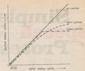
Fig. 2 Transfer characteristics for various degrees of amplitude limiting
