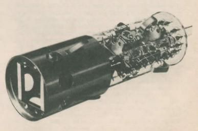
Fig. 9. Electrode assembly of Brimar mesh p.d.a. c.r.t. type D13–51GH (courtesy Thorn Brimar Ltd.)
