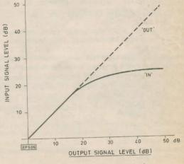
Fig. 10 Transfer characteristic
