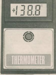
Precision Digital Thermometer; -55°C to +150°C; stainless steel probe; laser trimmed i.c. sensor giving excellent linearity and easy calibration. ... These will be followed in the June and July issues by at least 6 more projects designed to fit in the case
