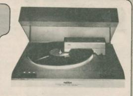
New Revox B795 direct drive turntable with Linatrak tangential tracking system. Motors are controlled by Hall effect sensors via quartzreferenced phase locked loops. *Courtesy Studer Revox America Inc.*
