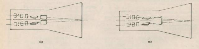
Fig. 8. (a) Dual-gun tube; (b) Dual-gun tube with common X- deflection plates (courtesy Enertec Instrumentation Ltd.)
