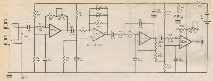
Fig. 5 Circuit of Speech Processor
