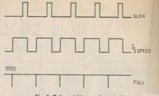
Fig. 1. Pulse width speed control
