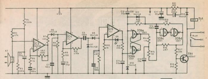
ing C13 via R14 and when the lower threshold of the Schmitt trigger is reached pin 4 goes low turning off TR1 and de-energising RLA. If relay RLA is removed and R21 linked TR1 can drive a low power high efficient piezo sounder such as the ITT U250-RHA which requires 12V d.c. at 18mA to produce a 105dB 2.7kHz at 1 metre.
