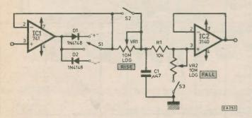
HIS circuit was originally designed for use in a' voltage-controlled synthesiser as a multi-purpose voltage processor, but it can be applied to many other uses.
