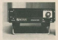
The unit which measures only  $100 \times 32 \times 120$ mm has a frequency range of 10Hz to 500MHz and can measure up to 500MHz with a prescaler. Powered by either 4 penlight batteries or an external d.c. supply (8 to 11V) the instrument has a 4 digit display and a resolution of 10Hz/10kHz with a maximum input of 20V.
