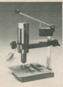
The senior model is supplied with an automatic 3-jaw chuck and a precision chuck with 5 collets is available as an optional extra (0.6, 1.2, 1.8, 2.4 and 3.2 mm).
