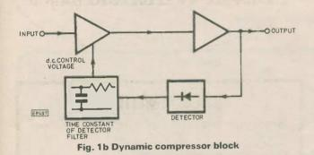
a certain threshold level. 'Soft-limiting' offers some advantages over 'hard-limiting' as regards the generation of unwanted harmonics of the input signal. These are considerably reduced with the result that the output signal is less harsh and consequently more pleasant to listen to. Also, due to the reduction in harmonic content, less stringent requirements are imposed on the subsequent filter stage. Typical signal waveforms obtained with 'hard' and 'softlimiting' are shown in Fig. 3.
