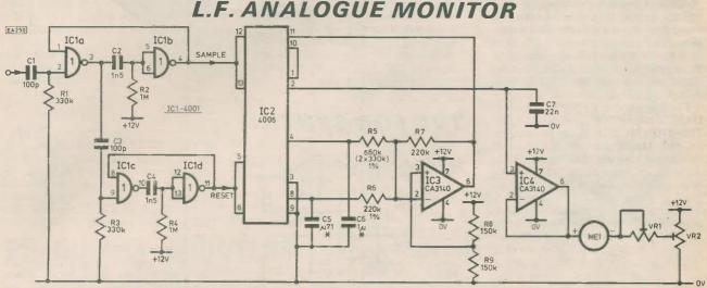
MOST low frequency measurements, e.g. the human pulse rate, involve a compromise between a slow response and a pulsating output. This can be avoided by calculating the reciprocal of the interval between pulses. Done digitally, this is elegant, but costly enough in itself to increase the pulse rate!
