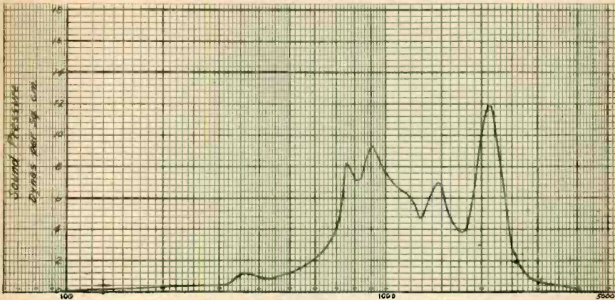
Fig. 4. Curve for 15 in. Conical Horn With 10 in. Opening and 90 Degree Bend.
