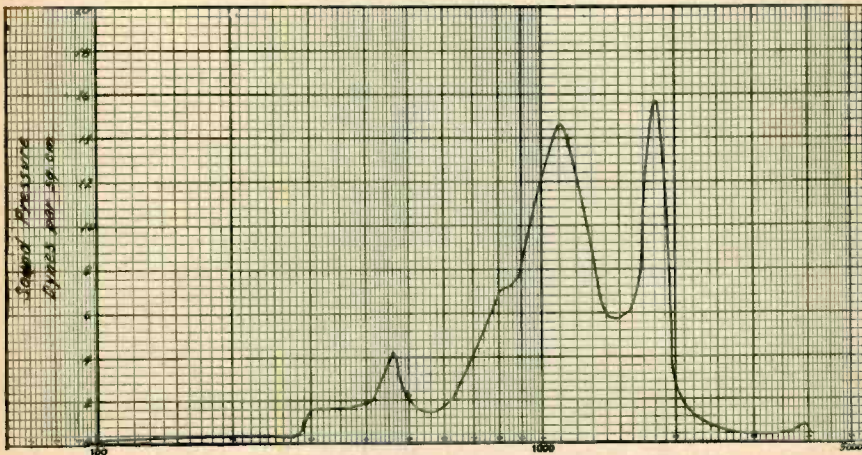
Fig. 5. Curve for 18 in. Exponential "Goose-neck" Horn With 10 in. Opening and Poor Unit.
