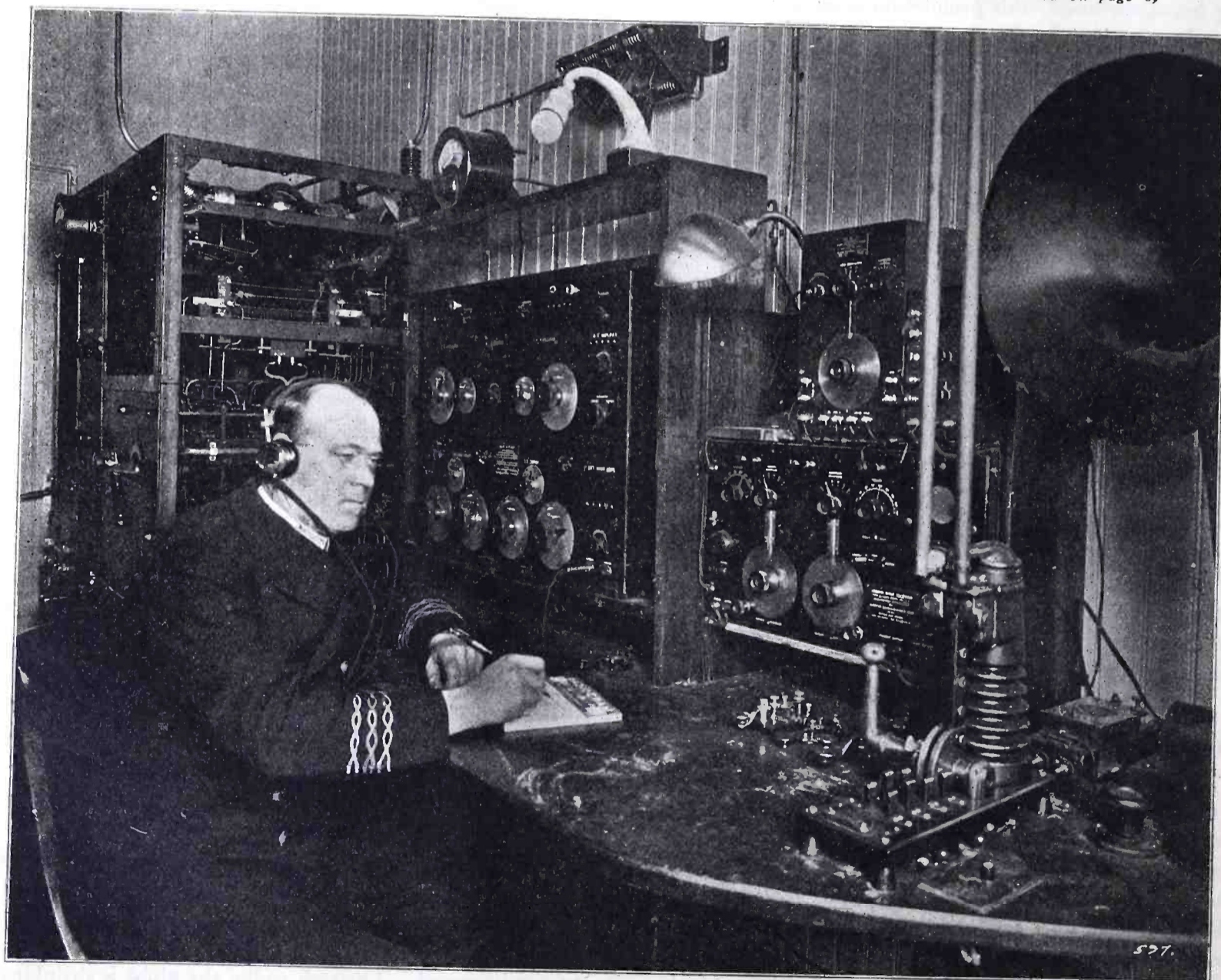
Radio Equipment on S.S. "Leviathan," Comprising Four Independent Transmitting and Receiving Outfits. The Main Transmitter is Equipped with Two 10 K. W. Tubes
