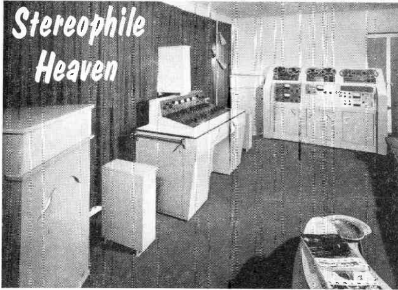
Howard Souther's Stereophile Heaven showing at far end of room two professional Ampex tape machines and one Magnecorder, used for duplicating and for various sound effects. Control console is at center of photograph.
