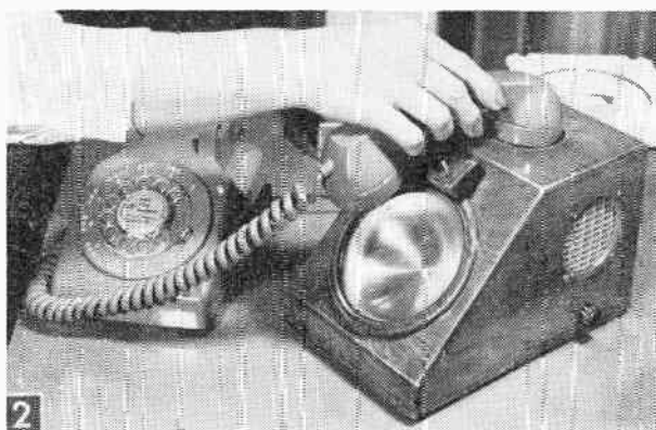
Placing the phone hand set in position on the amplifier cabinet when receiving or making a call automatically turns on amplifier switch.
