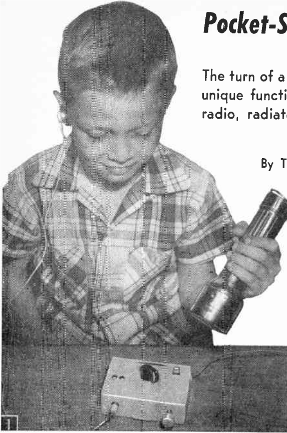
The 3-in-1 Transistorlab with switch in A-position functions as a solar-powered radio, here being activated by the beam of a flashlight.
