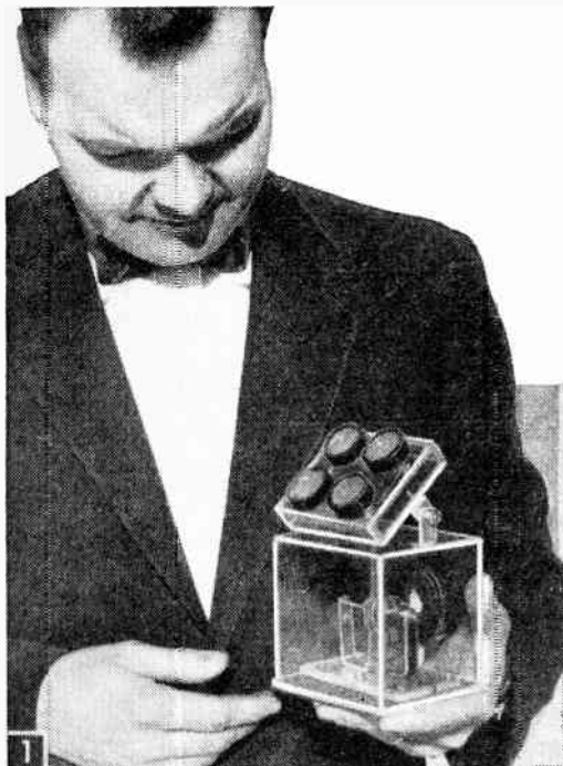
Four black discs on top of case (Fig. 2) are silicon solar cells that convert sunlight into electricity to operate motor enclosed in plastic case. Note whirling fan blades in Fig. 1 that indicate motor is running from electricity generated by solar cells.
