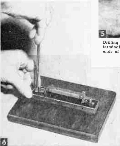
6 Roundhead wood screws fasten the Bakelite base piece to the wood base, through holes bored in the ends of the Bakelite.
