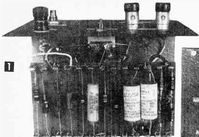
A compact and efficient unit designed for continuous service—a transistorized capacitor relay, front-panel and under-chassis views.
