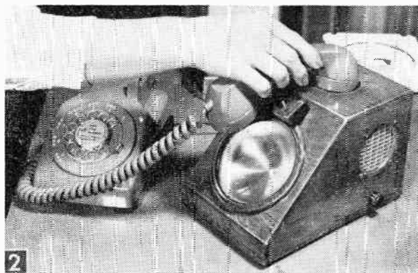
Placing the phone hand set in position on the amplifier cabinet when receiving or making a call automatically turns on amplifier switch.
