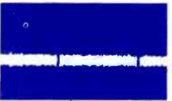
14. COLLECTOR, 1st BANDPASS AMPL., (Q13), BURST 8V P-P, CHROMA 4V P-P, HORIZ. (PWS1)
