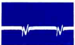
17. COLLECTOR, 2nd BANDPASS, (Q14), 0.22V P-P, HORIZ. (PWS1)
