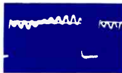
25. OUTPUT G-Y AMPL., V4, TPF3, WITH COLOR, 150V P-P, HORIZ. (PWS2)
