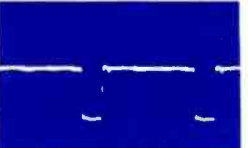
22. OUTPUT R-Y AMPL. V4, TPF2, NO COLOR, 90V P-P, HORIZ. (PWS2)
