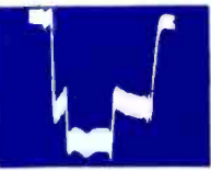
④ 1.9V P/P, 15,750Hz Hor. Sync. Pulse Showing 4.5MHz Trap out of Adj.
