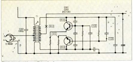
Fig. 8 A typical bias oscillator circuit.
