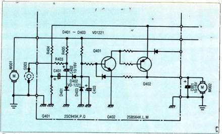
Fig. 5 A typical auto shutoff circuit.
