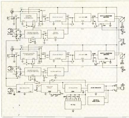
Fig. 6 A block diagram of a typical tape recorder.
