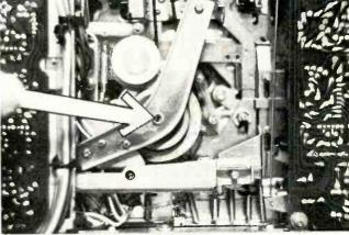
Fig. 4 Flywheel clearance adjustment.
