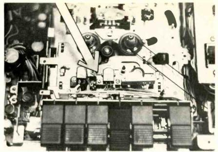
Fig. 9 Play/record head alignment screw.
