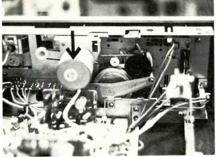
Fig. 1 Front load cassette transport. Motor indicated.
