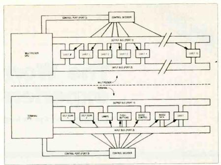
Fig. 2 Internal hardware architecture of IDAC/15 components. Input and output buses are created with I/O ports, and a third port controls device behavior. Interconnection between these two systems is a pair of current loops from UAR/T to UAR/T.
