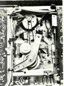
Fig. 2 Top load cassette transport mechanism.
