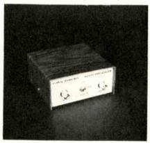
involved in tone signaling, tone activated squelch, etc. The PS-2 consists of a voltage controlled oscillator operating at 10 or 100 times the input frequency phase-locked thru divide by 10 or divide by 100 dividers. The unit evaluated by ET/D lived fully up to specifications but noticeably had rather little range beyond them. Its sensitivity is 25 mV and its output is 6V p-p, adequate for, and compatible with, almost any counter. The price of the PS-2 is \$39.95 assembled; \$29.95 as a kit.
