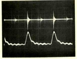
Fig. 4--The proper timing of the color burst and keying pulse is shown in the oscillograph waveform. The top trace is color burst information at V16 burst amp plate, while the bottom trace is simultaneously compared with the keying pulse at pin 2 of the same tube.
