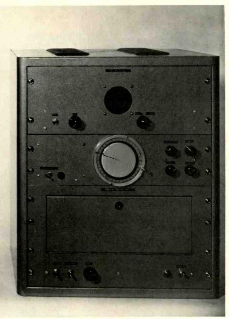
Cathode ray tube lightning detector (Courtesy British Columbia Forest Service)
