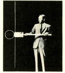
gulation, the direction from which noise impulses are being propagated along any given power line. The unit pinpoints sources of interference to TV and communications reception. Price \$595. International.
