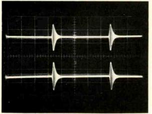
Fig. 5--The dual-trace oscilloscope waveform shows a balanced 3.58MHz color burst signal taken at the secondary of the AFC and ACC phase detector transformer.
