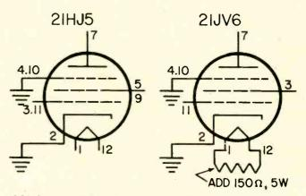
13GB5 tube, which replaced the 21HJ5 in later runs of these chassis, has been suggested as a substitute. However, this substitution required changing the tube socket and other components. We can now supply the 21JV6 which will replace the 21HJ5 with only slight rewiring of the original socket and the addition of a resistor across the heater.
