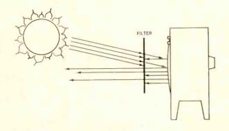
Fig. 3-A 50 percent transmission filter demonstrates how only 25 percent of the reflected light is seen but 50 percent of the phosphor light is seen. to the TV set as shown in Fig. 3.
