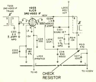
toms are noted. Sometimes the failure of the 6JC6A 3rd video IF tube will result in failure of the plate/screen load resistor, R213. Check the condition of this  $470\Omega$ ,  $\frac{1}{2}$  w resistor when replacing a defective 6JC6A tube.
