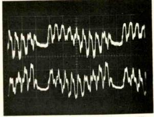
Fig. 7-The dual-trace waveform shows the color difference signals of -(B-Y) top waveform and -(R-Y) bottom waveform which will appear at terminals eight and nine of the IC demodulator.
