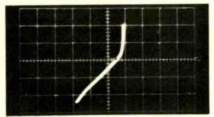
Fig. 13--Waveform showing transistor with base to collector leakage.
