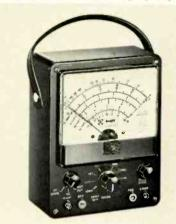
100, 500 and 5K; ac-dc current at 0-1, 10, 100ma, 1a; ohms at 0-5K, 50K, 500K and db readings from -20 to +76db in six ranges. The unit measures 6¾ in. x 5¼ in. x 2¾ in. and comes with a battery, test leads, carrying strap and operating manual. Price is \$19.95. Allied.
