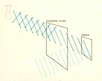
Fig. 6--When light is reflected from a smooth surface, the angle of polarization is not reversed.
