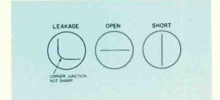
Fig. 4--Three basic waveforms produced by a defective transistor.
