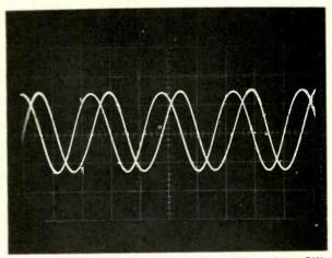
Fig. 8-- A dual-trace triggered scope waveform of the CW signal. The 3.58MHz CW signal had been superimposed on the scope for an exact phase check of the 104deg signal shift.
