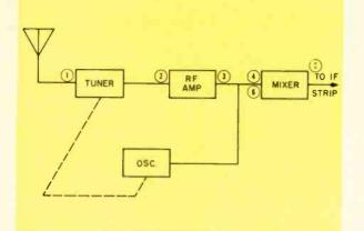
Fig. 8--Block dlagram of typical TV RF section.
