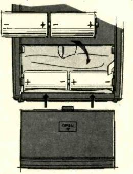
battery outline provided on the plastic pull-out tab. This will result in jamming of the tape in the PLAY OF RECORD positions.
