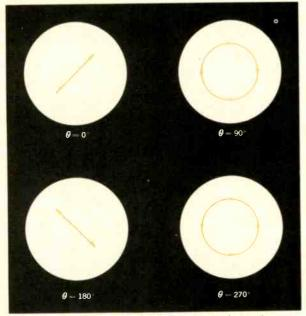
Fig. 8-Patterns formed on the scope are dependent on the phase relationship between the horizontal and vertical sinewaves.
