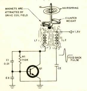
circuit to drive the clock mechanism. The transistor clock circuit closely resembles a blocking oscillator. In place of *Continued on page 88*
