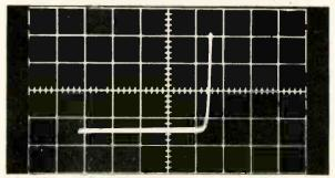
Fig. 10--Actual oscilloscope waveform showing a good transistor with probes connected from emitter to collector.
