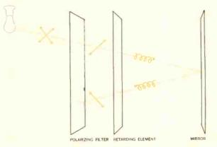
Fig. 10--The phase shift of light in the retarding element permits the virtual elimination of reflected light in the linear polarizing filter.
