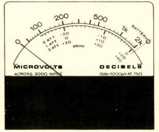
Fig. 1--Typical signal strength meter face reads dbmv and microvolts.
