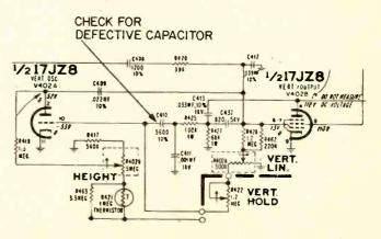
production models, connected to the vertical oscillator grid.
