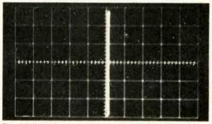
Fig. 11--Waveform showing a shorted transistor.
