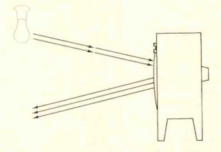
Fig. 2--When the set is turned on, light from the phosphor overpowers the reflected light and makes the screen appear black.
