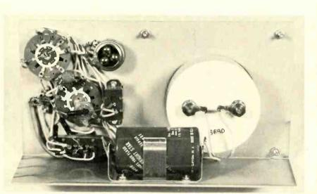
Model IT-18 in-circuit/out-of-circuit transistor tester measures gain (beta) and leakage. The circuit is basically a low impedance, common-emitter amplifier using the transistor being tested to complete the circuit.
