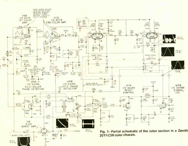
proper timing of the color burst and keying pulse in this stage is shown in Fig. 4, oscillograph wavetrace. The top trace is color burst information at V16, burst amp plate pin 7, while the bottom trace is simultaneously compared with the keying pulse at pin 2 of the same tube.
