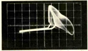
Fig. 14--A weird looking waveform taken from emitter to collector of a good transistor with inductance and capacitance in circuit.
