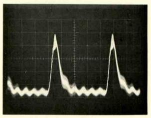
Fig. 2--A normal color burst signal taken from pin 2 of the burst amplifier tube.
