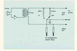
Fig. 8--Schematic of the transistor or diode tester.
