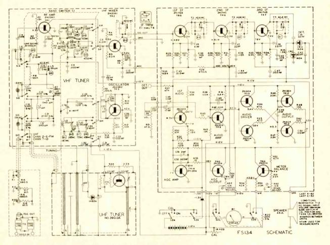
Fig. 4--Schematic diagram of SSM Model FS134 (Courtesy of Sencore).
