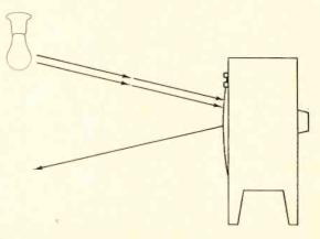
Fig. 1--Reflected light allows you to see the screen when there is no light from the set itself.
