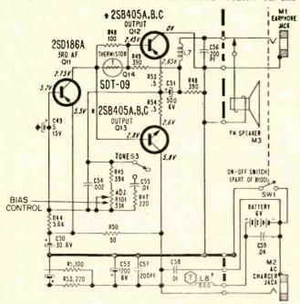
circuit board just to the left of the speaker magnet. If the control is defective, moving it usually causes the distortion to be intermittent. The problem is a poor connection where the lug is riveted to the control element—we suggest replacement of the control. The replacement control must be adjusted according to the procedure given in service manual S1214—if it isn't, you may still have distortion or high current drain.
