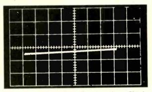
Fig. 7--A normal waveform taken from the emitter to collector of transistor.
