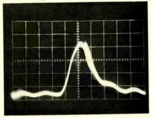
Fig. 3--An improper color burst signal waveform expanded for detail. The 3.58MHz burst signal is shown riding on the side of the keying pulse.
