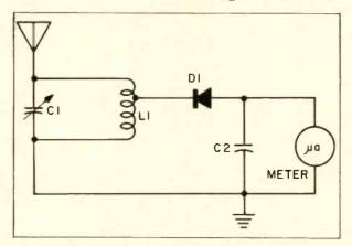
Fig. 2--Simplified schematic diagram of SSM circuit.
