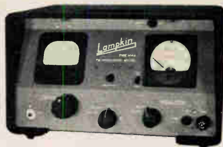
Lampkin type 205A FM modulation meter.
