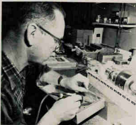
Robert Hutches, Anderson technician, soldering base plate of model T99 translator.
