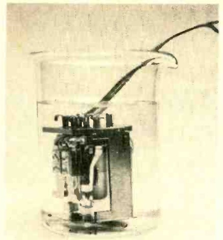
Relay being operated while submerged in 'Freon' TF.
