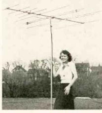
channel section, both being coupled for 300-ohm termination. A sharp horizontal pattern with superior front-to-back ratio minimize ghosts and interference. Reinforced construction uses drawn aluminum elements with crimped ends. LaPointe Electronics Inc., Rockville, Conn.— TECHNICIAN.
