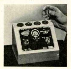
tester uses an electronic eye to reveal control-grid emission, also to indicate high resistance grid-cathode or cathode-heater shorts. Maker recommends it for checking tubes in the audio, i-f, and sync sections, where trial-and-error, wait-and-see substitutions are normally used. List price, \$24.95. Available in kit form as model GCT-2, \$19.95. Seco Mfg. Co., 5015 Penn Ave. S., Minneapolis, Minn.—TECHNICIAN
