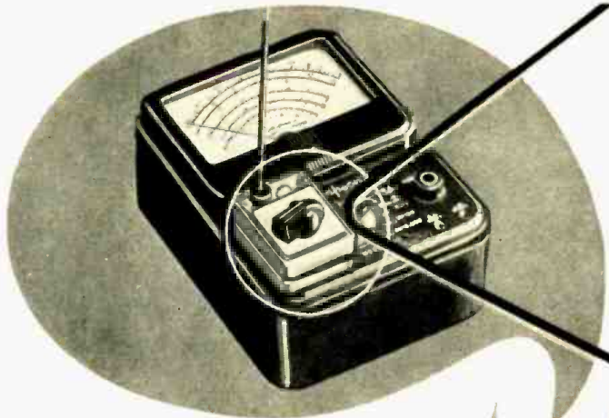
The adapter in place on the author's Simpson 260 meter and close-up of the adapter unit.
