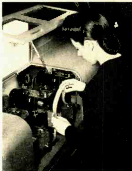
Punched paper tape, such as that which is shown in the photo in use in the famous Bell Relay Calculator, was the source of Harvard Mark I's instructions and programming.
