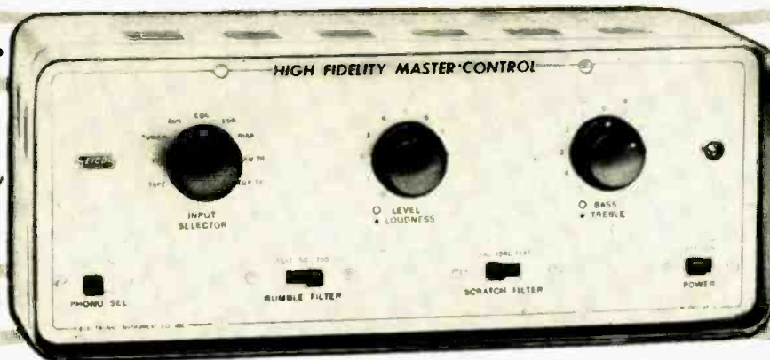
Front panel view of high fidelity control unit. Dual controls are used to simplify appearance.
