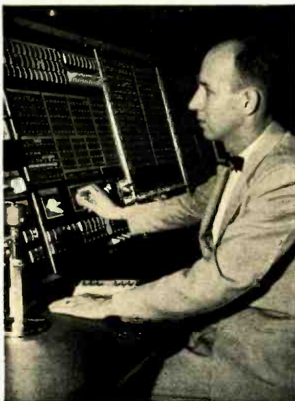
Miles does diagnostic programming on the Maintenance Console of the Sage Computer
