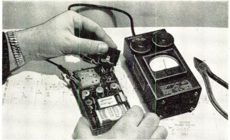
Fig. 3. The use of a battery-operated oscillator will avoid hum and noise pickup from the a.c. line. The receiver shown under test is the Regency transistor radio.
