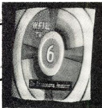
Fig. 1. Case of reduced width accompanied by pincushioning is shown left. This occurred in an Olympic Model DX-214 TV receiver and was caused by a defective width coil shown below, and misadjusted picture tube corrector magnets for the yoke.
