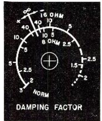
The Bogen Models DB20DF and DO30A both of which incorporate the variable damping factor control. (Right) Calibration.
