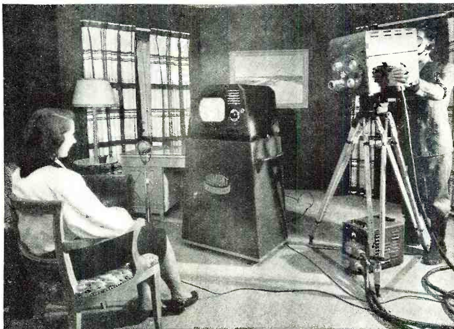
Fig. 3. View of remote position showing camera and receiver operating.
