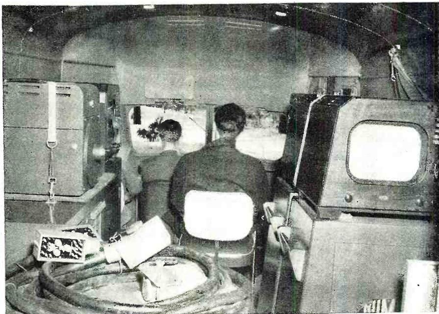
Fig. 2. Front interior view shows traveling accommodations for driver and the two operating personnel. TV receivers are at right, camera at left.
