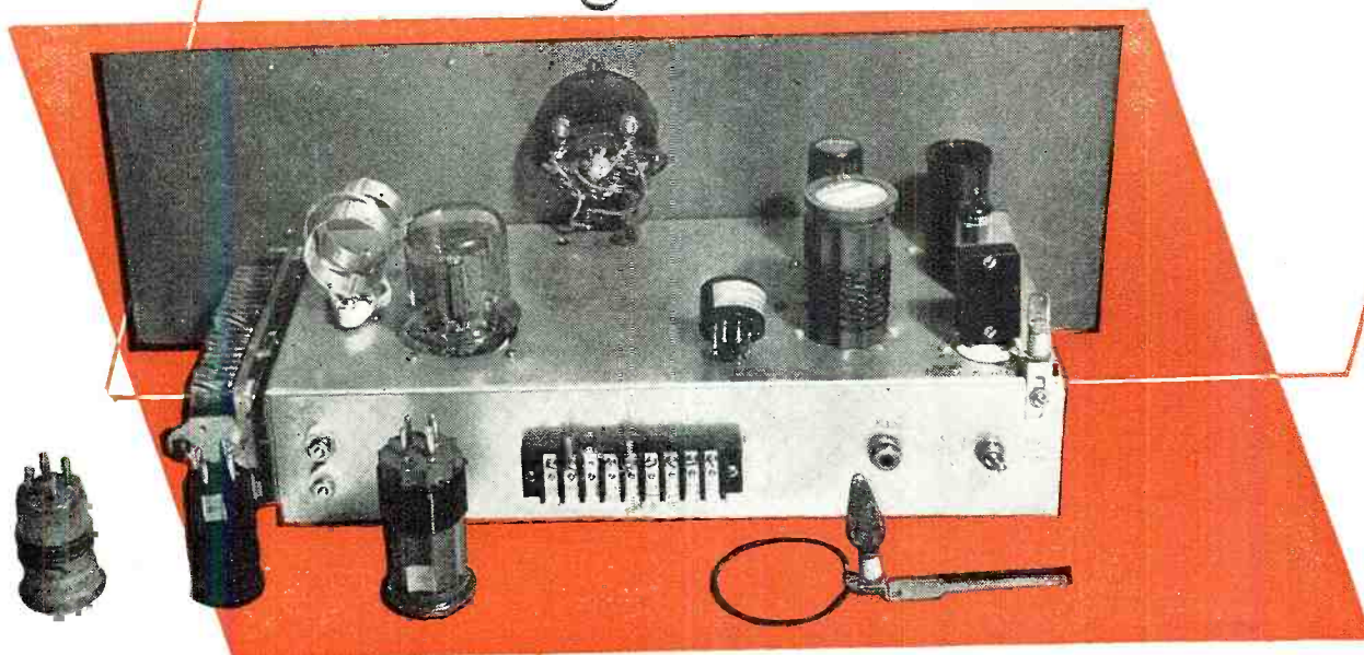
Fig. 1. Rear view of the three-tube transmitter, capable of operation on all bands from 10 through 80 meters, which uses an 826 as the final amplifier.
