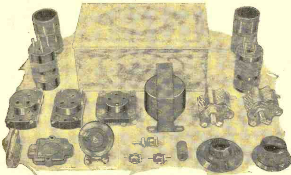
The parts before assembly: below, left to right, grid leak, grid condenser, rheostat, pin jacks, knobs; center, tube sockets, transformer, condensers; rear, coils, candy box.
