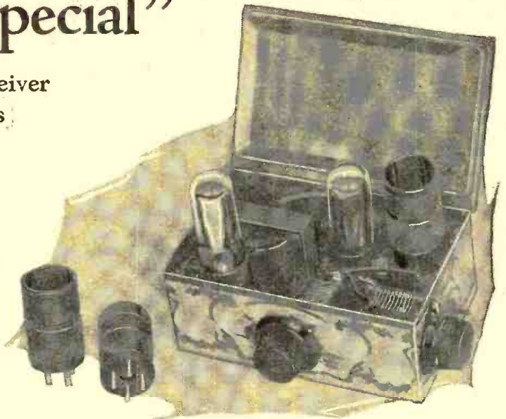
The completed "Candy-Box" Special receiver set up for operation, with a plug-in coil and the two tubes in place. Two of the other coils are shown at the left of the box itself.
