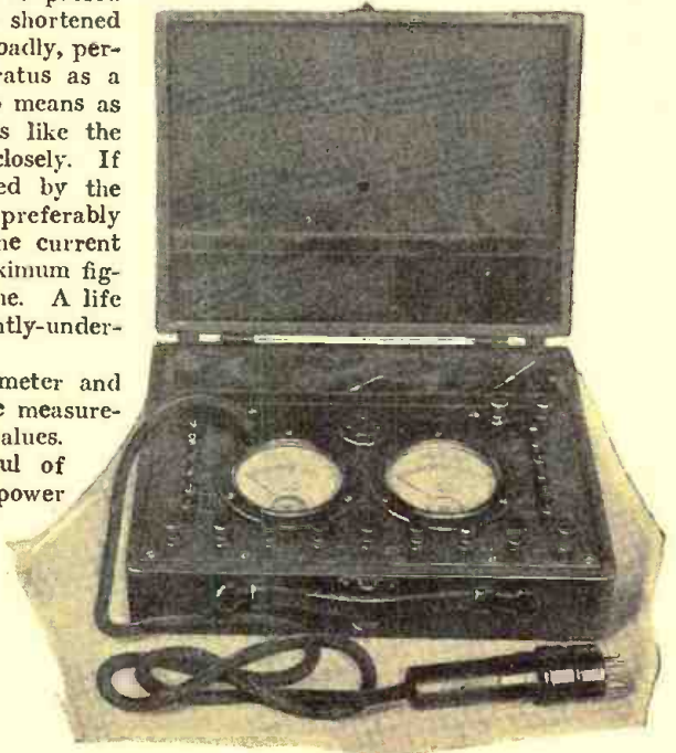
Another high-grade all-purpose instrument, the Jewell. The meters are thrown in and out of the circuit by means of small push-buttons. With the plugs, readings are taken at the sockets.
