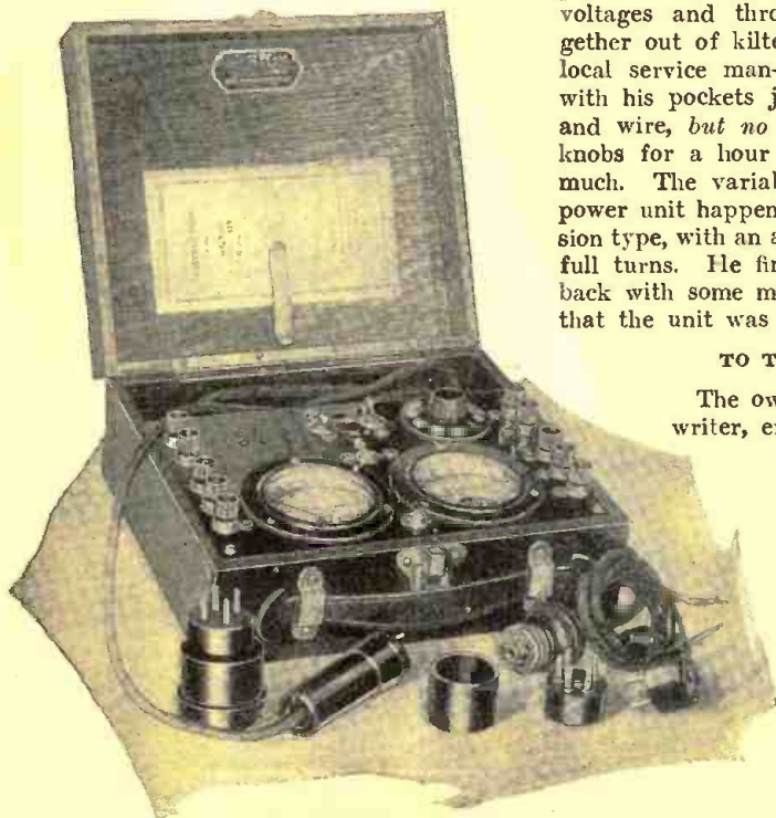
Worth its weight in gold—the Weston A.C.-D.C. test set. This is equipped with a rotary switch which makes the two meters read every current and voltage value in a receiver.
