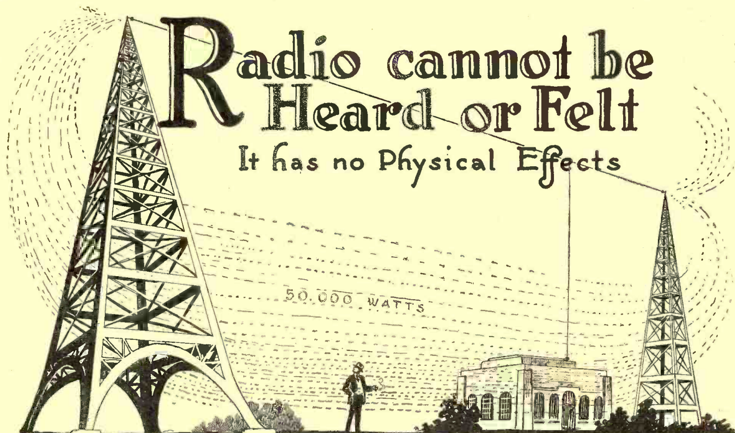
Beneath the aerial of a 50-kilowatt station which is transmitting, a piece of insulated metal (like an automobile body) quickly gathers an electric charge out of the magnetic field. But a human body does not; nor can the man in the midst of this field tell when it is turned off.
