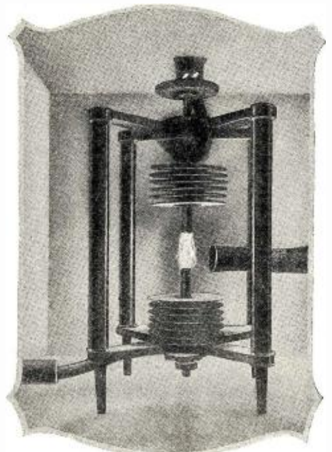
Shades of old time interference! The old DeForest spark gap at the Manhattan Beach station.
