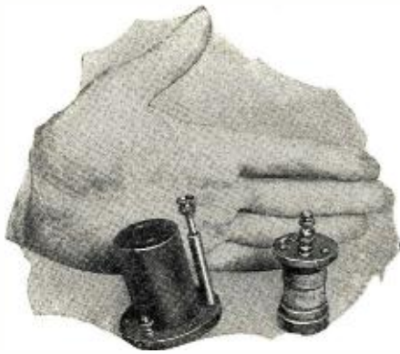
The essential parts of the radiation eliminator.
