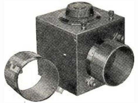
An inductance and variable condenser comprise a unit which can be used as wavemeter or wave-trap.
