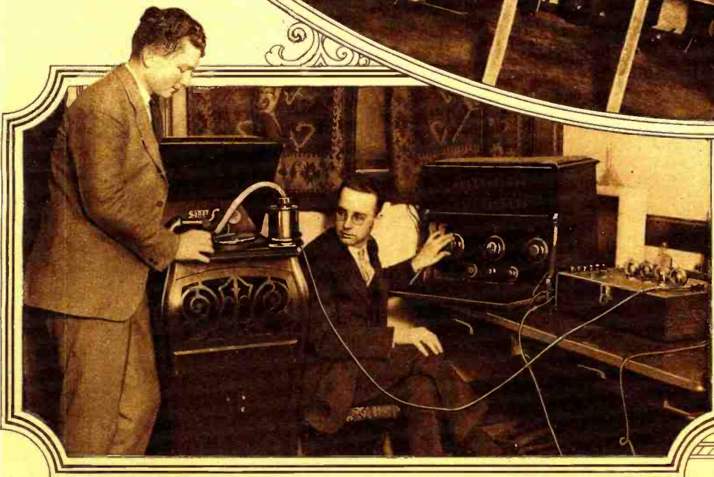
DEVICE FOR RECORDING RADIO SIGNALS. Left. In the research laboratory of New York University, Messrs. Borden and Busee have recorded local broadcast concerts on phonograph records with the aid of their device. A special type amplifier is shown carrying the music to the loud speaker unit on the phonograph. © Kadel & Herbert
