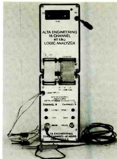
When the digital-storage-oscilloscope module is hooked up to the logic analyzer, your setup will look like this. The combined instruments make an almost unbeatable pair for testing and troubleshooting both digital and analog circuits.
