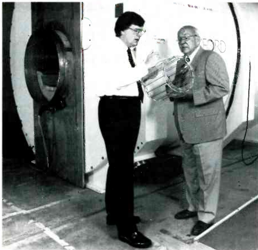
EXPERIMENTAL MAGNETIC RESONANCE SCANNER based on a 50-ton superconducting magnet, has twice the power of any used now, producing a uniform magnetic field of 4 Tesla in its 1-meter bore. Drs. John F. Schenck (left) and Rowland W. Redington are shown examining a coil used in making 4-Tesla magnetic resonance images of the head.
