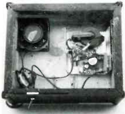
FIG. 5—THE PROTOTYPE'S BASE is made of wood. Holes are drilled in the front and rear for ventilation. Air movement is generated by the small fan mounted in the upper left corner.
