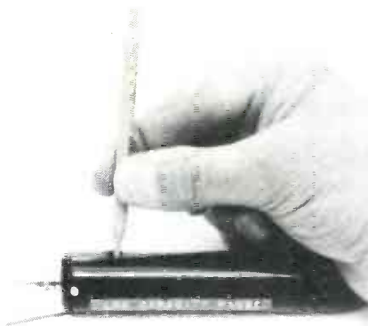
FIG. 8—ADJUST C1 USING an insulated tool for an optimum square-wave scope display.
