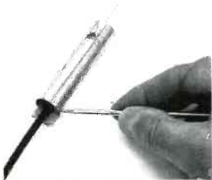
FIG. 4—THE POINTER INDICATES where the wiring board's solder lug is tack-soldered to the inside of the shield tube.
