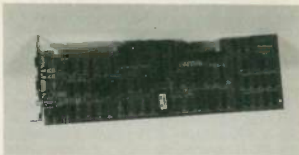
FIG. 1—THE QUADLINK IS A COMPLETE COMPUTER SYSTEM with its own CPU, disk controller, and RAM. It takes up only one PC expansion slot.
