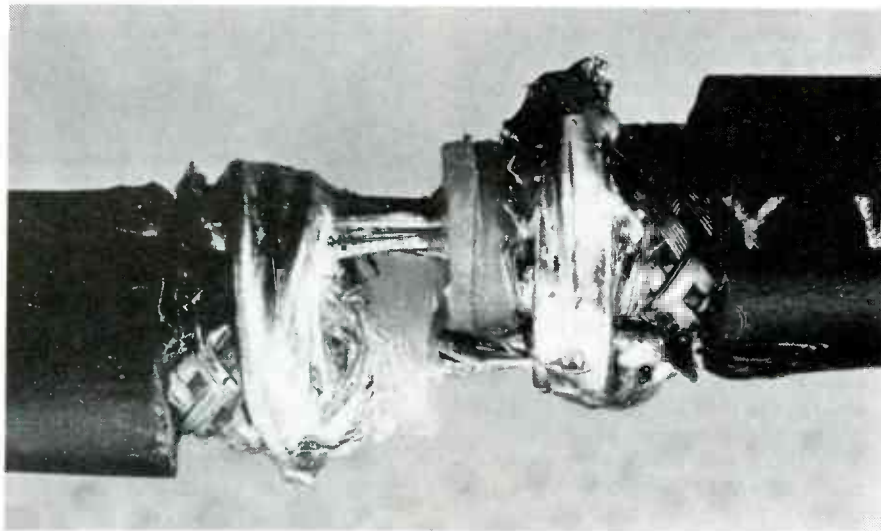
FIG. 14—FINISHED JOINT: Note that the center conductor is placed on the braid and braid ends wrapped around to secure conductor in place before soldering.
