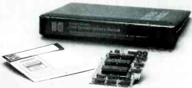
THERE ARE MANY double-density disk upgrades for the Model 1 , including this one from Radio Shack itself.
