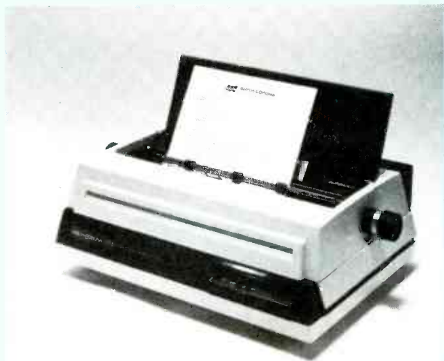
THE SMITH-CORONA TP-1 was one of the first low-cost, bidirectional daisywheel printers for personal computer use.
