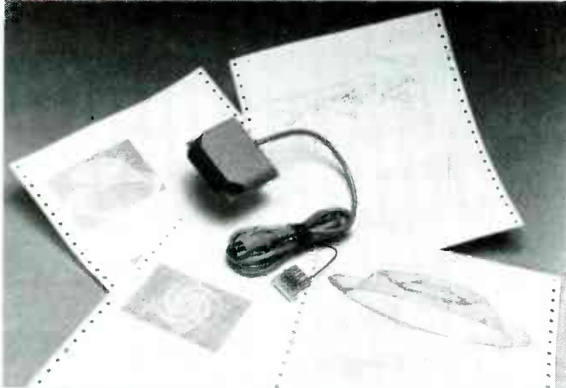
PRINTER INTERFACE , the Card/? from Cardco (313 Mathewson, Wichita, KS 67214) lets you use a Centronics-type printer with a Commodore computer.
