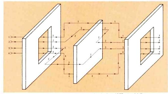
FIG. 2—SPEAKER BACK-WAVE is alternately combined and separated as it passes through and around SAFE enclosure's batfles.
