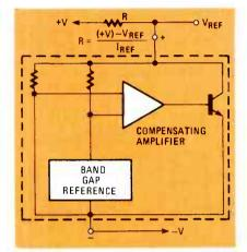
FIG. 6—THIS TWO-TERMINAL REGULATOR from Ferranti Electric can be used just like a Zener diode. It has a stability as great as 10 ppm per 1000 hours of operation.
