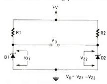
FIG. 3—THIS CIRCUIT shows one way to overcome the problem of temperature drift in Zener diodes.
