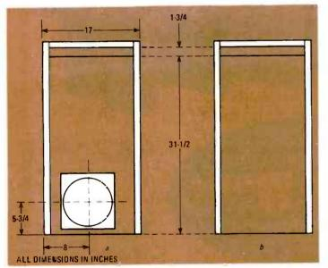
FIG. 9—SPEAKER SHOULD BE MOUNTED slightly off-center to prevent standing waves. Center figure shows distance between partition 1 and top of enclosure.
