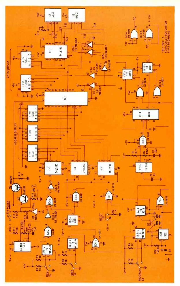
FIG. 1—WHILE ONLY R17 IS SHOWN, resistors R17-R24 are connected from the eight output-lines of S1 and S2 to ground.
