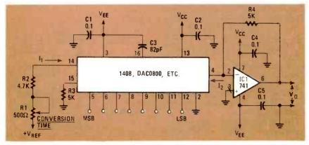
FIG. 12—A DIGITALLY SELECTABLE voltage reference. Once the input current ( $I_1$ ) to the D/A converter is set, the output from the circuit ( $V_0$ ) is determined by digital input (pins 5-12) to the D/A converter.
