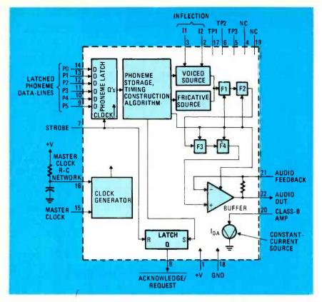
FIG. 4—VOTRAX'S SC-01 is a single-IC, phoneme-type, speech synthesizer intended for computer control.
