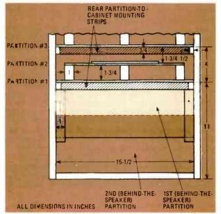
FIG. 5-NON-PERSPECTIVE VIEW from front of enclosure. Note construction of partition 1/partition 2 assembly.
