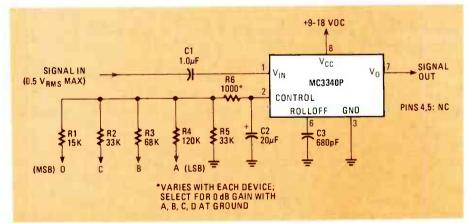
FIG. 2—SCHEMATIC DIAGRAM of a digitally-controlled attenuator circuit. Lines A, B, C, and D, can be driven by the simple circuit shown in Fig. 4.
