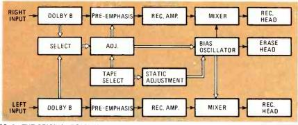
FIG. 2—THE ORIGINAL DOLBY HX system is shown in this block diagram. For the system to work, a control signal that is sensitive to amplitude and frequency content is required.
