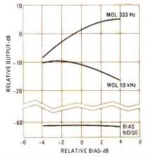
FIG. 1—THE BIAS LEVEL that provides the highest output with acceptably low distortion for a 333-kHz tone is quite different than the bias level required by a 10-kHz tone.
