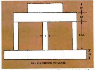
FIG. 11—SIDE VIEW of even-numbered partition mounted atop odd-numbered partition using partition mounting strips. Each strip is located as shown in Fig. 10 and measures  $1 \times 1 \times 134$  inches.
