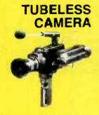
Video cameras have entered the all-solid-state age in the United States with the start of marketing of Hitachi's MOS camera, which uses a single <sup>3</sup>/<sub>2</sub>-inch metal oxide silicon IC as an image sensor. The MOS sensor has 180,000 picture elements, providing a claimed 260-line horizontal resolution. The camera weighs 3.96 pounds.
