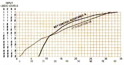
FIG. 3—NET CONTROL RESISTANCE and calculated attenuation plotted against four-bit control signals. Note that the calculated attenuation curve is nearly, but not quite, linear.
