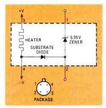
FIG. 5—A ZENER DIODE and an on-chip heater element are combined in the LM-199. The resulting IC is a highly stable voltage-reference device.
