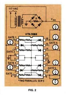
drivers. When using multiple SCR's and a common  $V_{AA}$  supply, gate-toanode leakage currents ( $I_{GA}$ ) can hold the supply voltage above the anode OFF voltage,  $V_{AK(OFF)}$ , and prevent proper turn-off. Resistor R is connected across the power supply to insure proper SCR operation.
