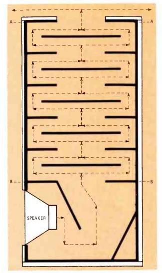
FIG. 1—SIDE VIEW OF SAFE ENCLOSURE showing speaker back-wave path. Path is symmetrical between points A and B.
