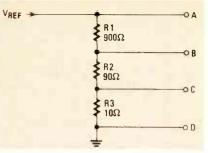
FIG. 11—A RESISTOR NETWORK can be used to get a multiple-output voltage reference. The voltage at each tap is 10 times higher than the voltage at the tap below it.
