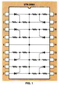
Characteristics of any individual SCR (maximum limits are given unless otherwise specified) are: Forward blocking-current. 50  $\mu$ A; gate-to-anode leakage. 250  $\mu$ A; forward ON-voltage. 1.2 volts at +25°C and 1.15 volts at +55°C; gate trigger-voltage. 2.5 volts; gate trigger-current. 300  $\mu$ A; gate OFF-current. 10  $\mu$ A; holding current, 10 mA at 0°C and 5.0 mA at +55°C, and anode
