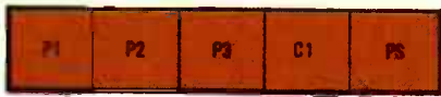
FIG. 12—FIVE-BYTE PREFIX carries information for multiplexing and error detection, and describes the data group that follows.
