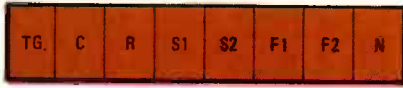
FIG. 13—DATA GROUP HEADER provides information concerning the treatment of the videotex data.
