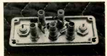
IF BANDPASS FILTER provides satellite TV receiver with the required selectivity. To find out the other missing components of the receiver, turn to page 47.
