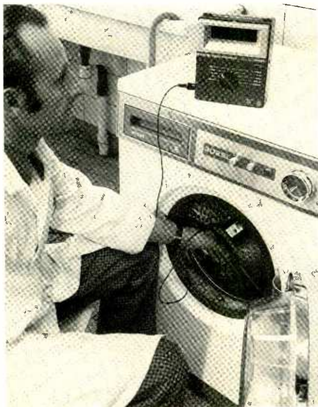
AN ACCURATE TEMPERATURE CHECK is necessary when servicing household appliances such as a clothes dryer
