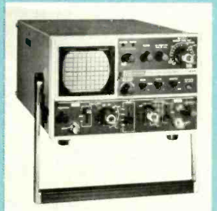
DUAL-TRACE oscilloscope, with bandwidth 15 MHz or more, is needed for VCR troubleshooting and adjustments.
