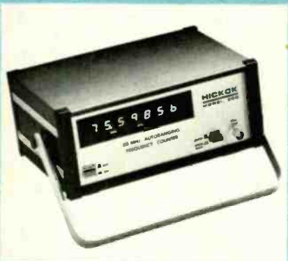
NEW TO TELEVISION servicing, frequency counter occupies important place in VCR troubleshooting.
