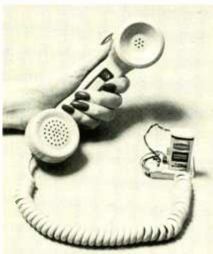
FIG. 1—ONE-STATION INTERCOM is powered by a 9-volt transistor battery and has an LED status indicator.
