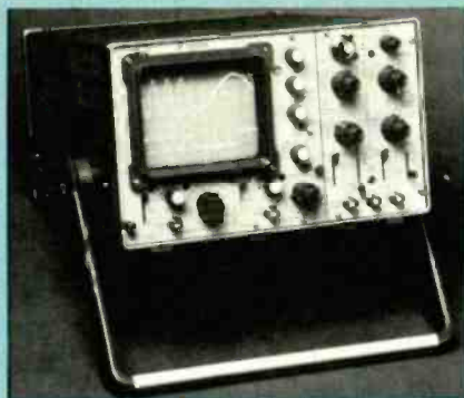
DELAYED TRIGGER feature in more expensive oscilloscopes enables viewing waveforms you could not otherwise display.
