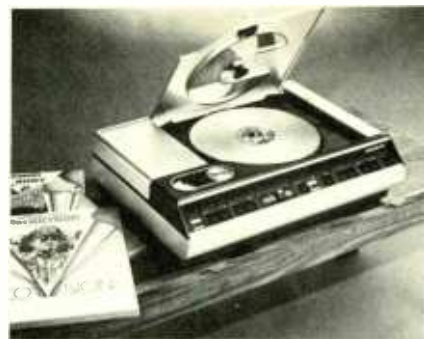
MAGNAVISION PLAYER WITH the lid up. The unit cannot be turned on until the lid is closed.
