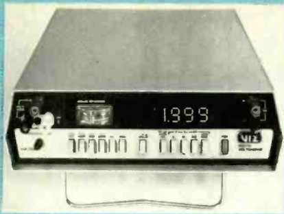
NARROW TOLERANCES of some voltages in VCR servicing recommend at least a 3½-digit multimeter.
