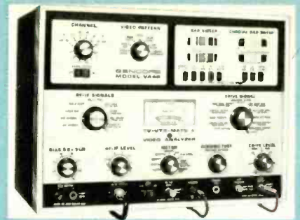
SENCORE INSTRUMENT has its own video and color bar patterns, plus multiburst for frequency response tests.
