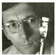
BELL LABS SCIENTIST prepares to test experimental two-layer gallium arsenide/aluminum gallium arsenide semiconductor crystal (shown to the right of the light). New crystal technique increases the speed at which electrons move through the crystal. Such a breakthrough in solid-state technology could lead to faster, more efficient semiconductor devices.
